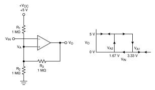
Figure 7-3. TLV1812-EP in an Inverting Configuration With Hysteresis
