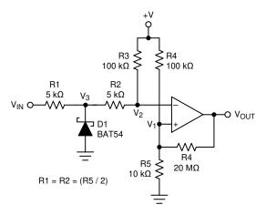
Figure 7-17. Zero Crossing Detector
