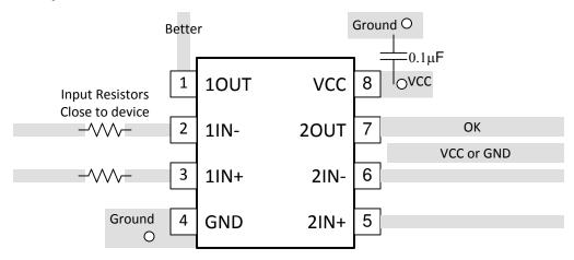
Figure 7-20. Dual Layout Example
