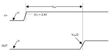
Figure 6-3. Power-On Reset Timing Diagram
