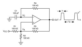
Figure 7-9. Square-Wave Oscillator
