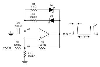
Figure 7-12. Adjustable Pulse Width Generator
