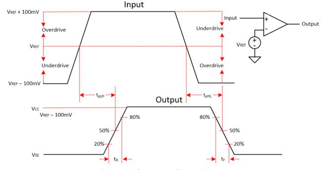
Figure 7-1. Comparator Timing Diagram
