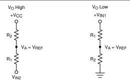
Figure 7-6. Non-Inverting Configuration Resistor Networks
