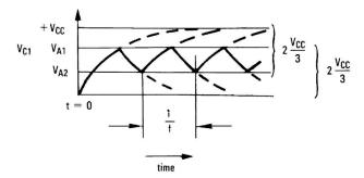
Figure 7-10. Square-Wave Oscillator Timing Thresholds
