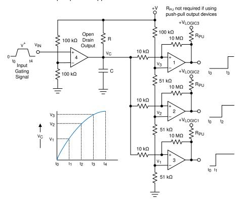
Figure 7-13. Time Delay Generator
