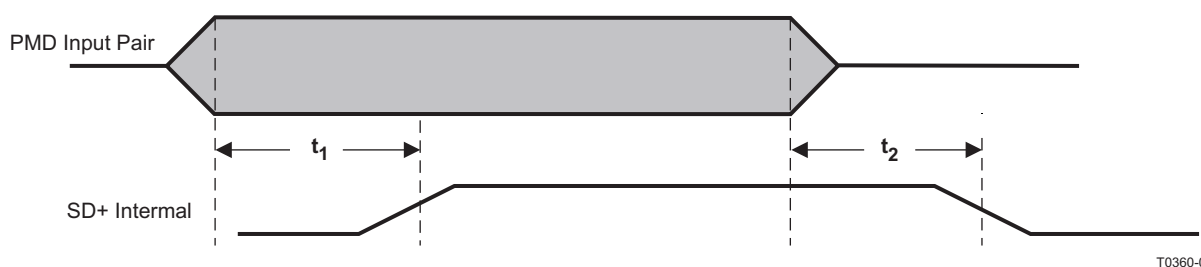
Figure 4-20. 100Base-TX Signal Detect Timing
