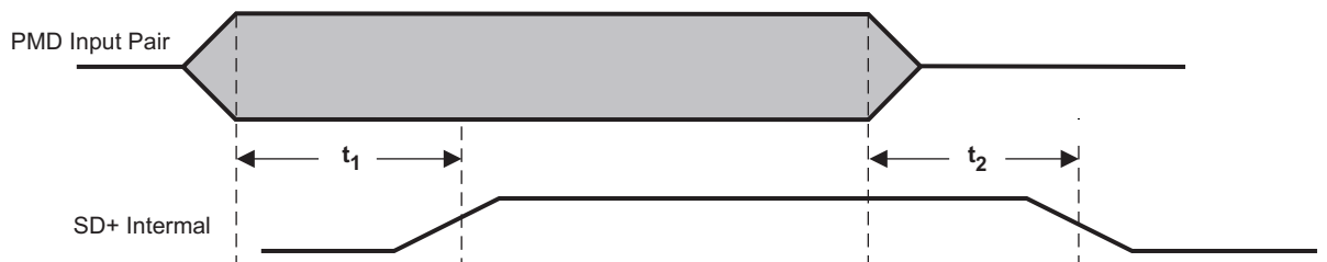
Figure 9-20. 100Base-TX Signal Detect Timing
