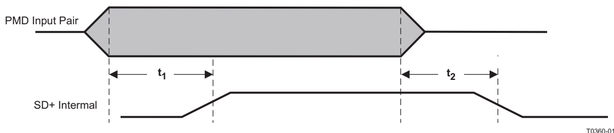
Figure 9-20. 100BASE-TX Signal Detect Timing
