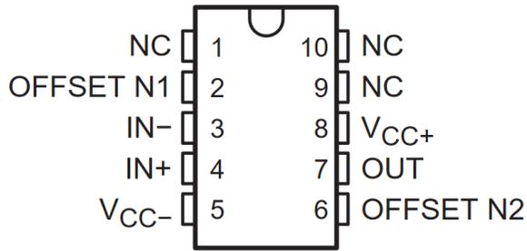
Figure 4-7. TLE2061 and TLE2061A U Package (Top View)
