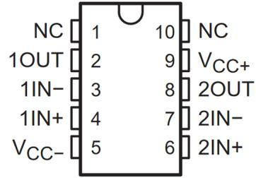
Figure 4-8. TLE2062 and TLE2062A U Package (Top View)
