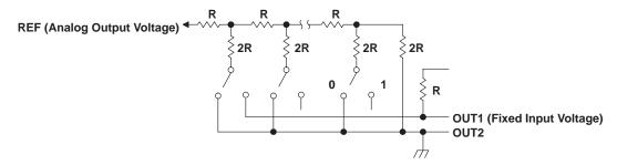
Figure 1. Voltage Mode Operation
