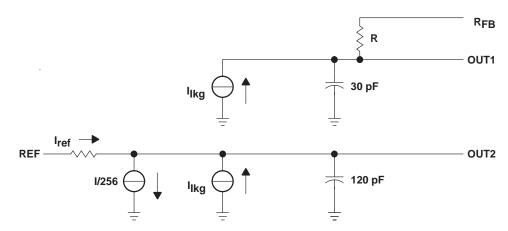
Figure 2. TLC7524 Equivalent Circuit With All Digital Inputs Low
