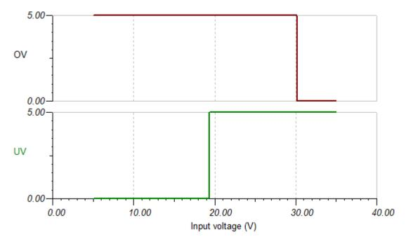
Figure 8-3. Window Comparator Results
