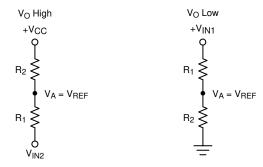
Figure 7-6. Non-Inverting Configuration Resistor Networks
