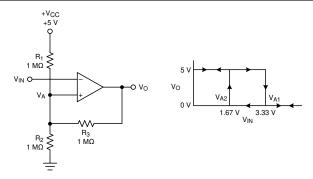
Figure 7-3. Inverting Configuration With Hysteresis
