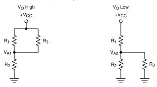
Figure 7-4. Inverting Configuration Resistor Equivalent Networks
