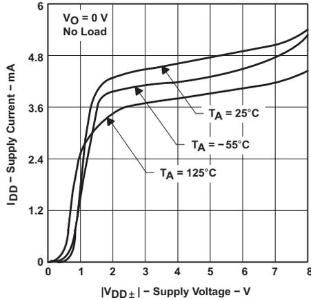
Figure 6-37. TLC2274-Q1 Supply Current vs Supply Voltage
