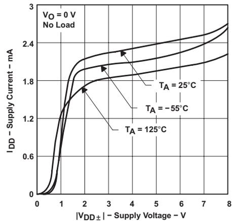
Figure 6-36. TLC2272-Q1 Supply Current vs Supply Voltage
