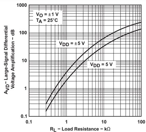
**Figure 6-24. Large-Signal Differential Voltage Amplification vs Load Resistance**
