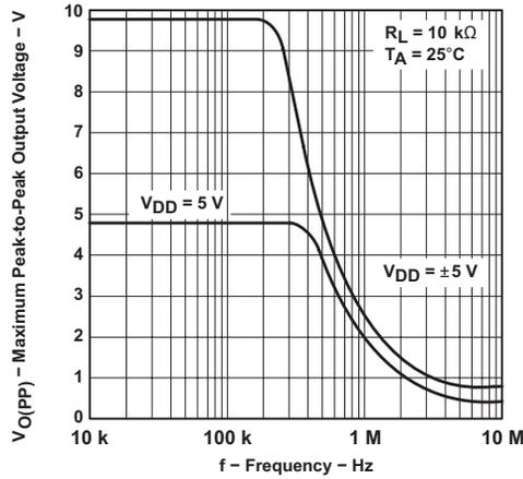
**Figure 6-19. Maximum Peak-to-Peak Output Voltage vs Frequency**
