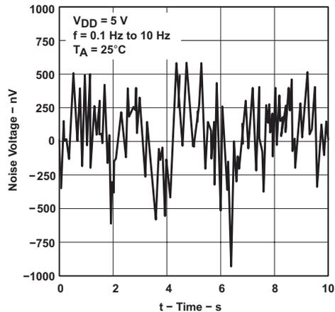
Figure 6-52. Noise Voltage Over a 10 Second Period
