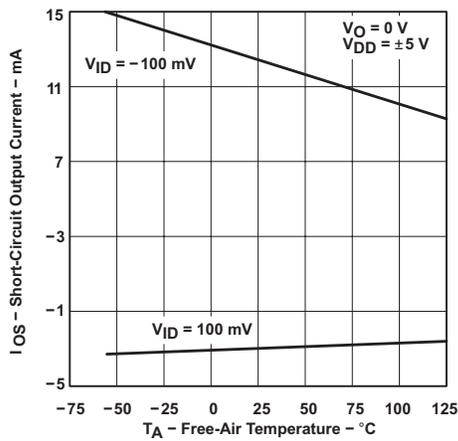
**Figure 6-21. Short-Circuit Output Current vs Free-Air Temperature**
