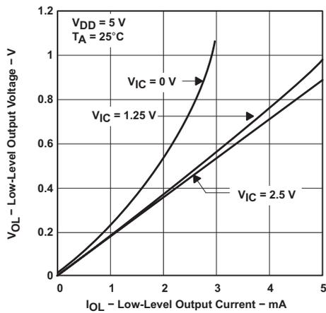
Figure 6-15. Low-Level Output Voltage vs Low-Level Output Current
