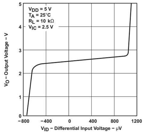
**Figure 6-22. Output Voltage vs Differential Input Voltage**
