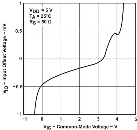
Figure 6-5. Input Offset Voltage vs Common-Mode Voltage
