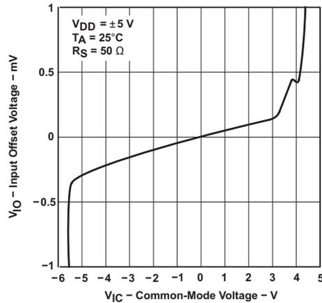
Figure 6-6. Input Offset Voltage vs Common-Mode Voltage
