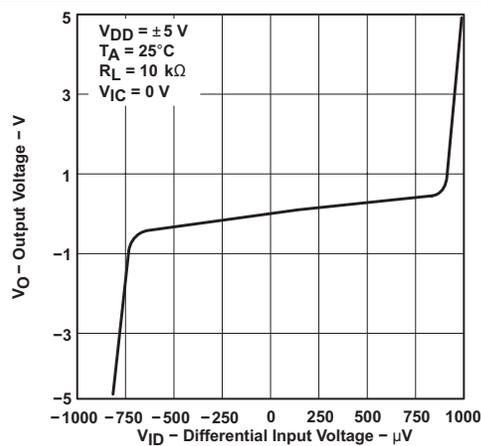
**Figure 6-23. Output Voltage vs Differential Input Voltage**
