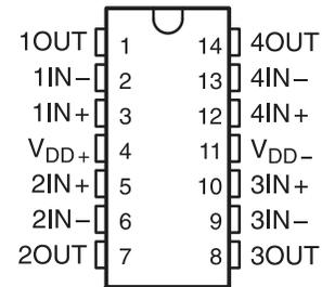
**Figure 5-2. TLC2274-Q1 and TLC2274A-Q1:
