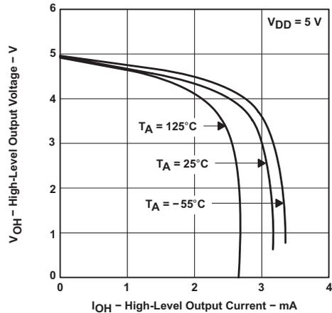
Figure 6-14. High-Level Output Voltage vs High-Level Output Current
