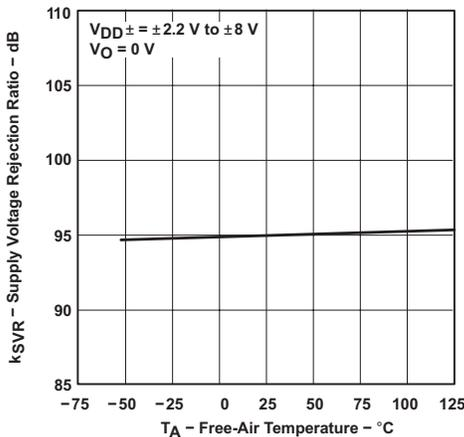
Figure 6-35. Supply-Voltage Rejection Ratio vs Free-Air Temperature
