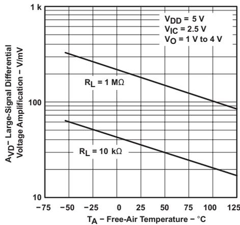
Figure 6-27. Large-Signal Differential Voltage Amplification vs Free-Air Temperature
