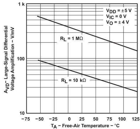
Figure 6-28. Large-Signal Differential Voltage Amplification vs Free-Air Temperature
