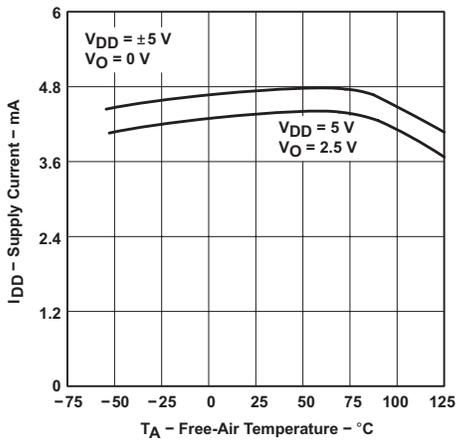
Figure 6-39. TLC2274-Q1 Supply Current vs Free-Air Temperature
