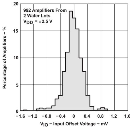
Figure 6-3. Distribution of TLC2274-Q1 Input Offset Voltage
