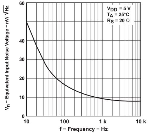
Figure 6-50. Equivalent Input Noise Voltage vs Frequency
