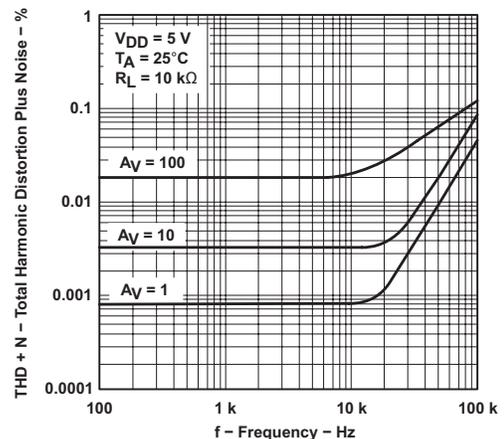
Figure 6-54. Total Harmonic Distortion + Noise vs Frequency
