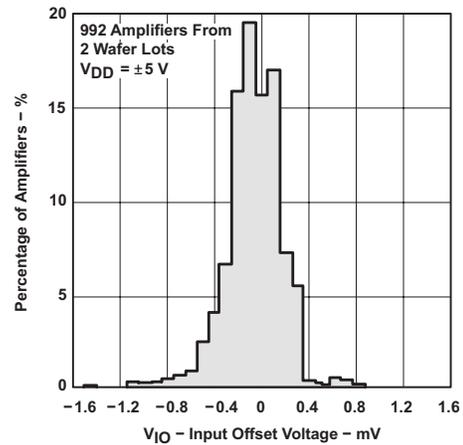
Figure 6-4. Distribution of TLC2274-Q1 Input Offset Voltage
