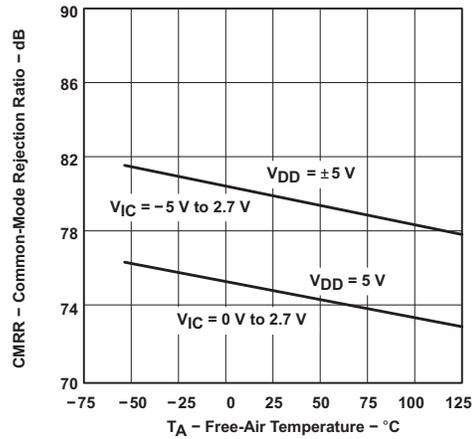
Figure 6-32. Common-Mode Rejection Ratio vs Free-Air Temperature
