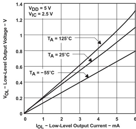
Figure 6-16. Low-Level Output Voltage vs Low-Level Output Current
