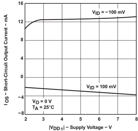
**Figure 6-20. Short-Circuit Output Current vs Supply Voltage**
