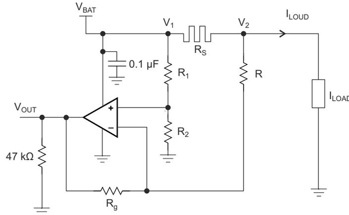
Figure 8-2. High-Side Current Monitor Equivalent Schematic (Each Amplifier)
