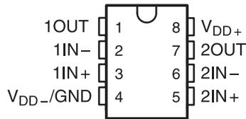
**Figure 5-1. TLC2272-Q1 and TLC2272A-Q1:
