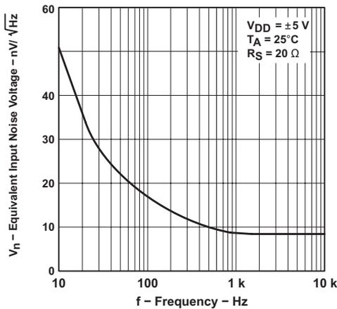
Figure 6-51. Equivalent Input Noise Voltage vs Frequency
