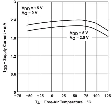
Figure 6-38. TLC2272-Q1 Supply Current vs Free-Air Temperature
