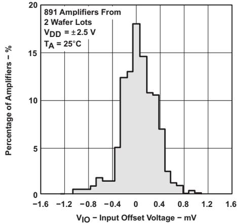
Figure 6-1. Distribution of TLC2272-Q1 Input Offset Voltage
