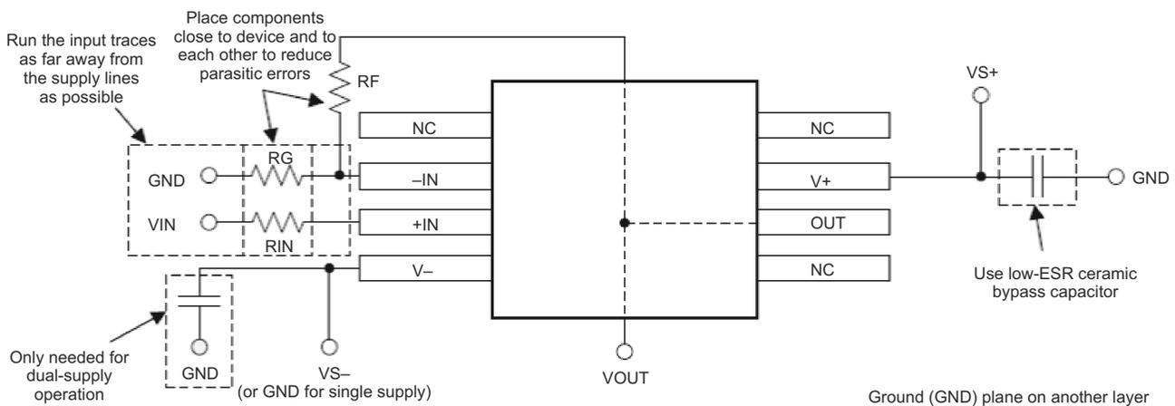
**Figure 8-6. Operational Amplifier Board Layout for Noninverting Configuration**
