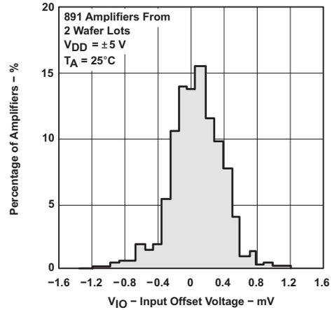
Figure 6-2. Distribution of TLC2272-Q1 Input Offset Voltage
