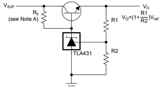
A.  $R_b$  is designed to provide cathode current  $\geq 0.2\text{mA}$  to the TLA431.
