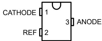
Figure 5-1. DBZ Package, 3-Pin SOT-23, TLA431 (Top View)
