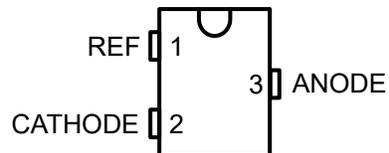
Figure 5-2. DBZ Package, 3-Pin SOT-23, TLA432 (Top View)
