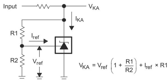
**Figure 7-2. Test Circuit for  $V_{KA} > V_{ref}$**
