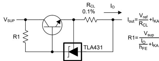
**Figure 9-9. Precision Current Limiter**
