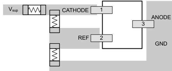
**Figure 9-11. TLA431 DBZ Layout Example**
