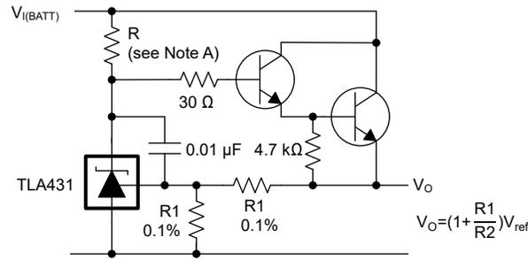
A. R is designed to provide cathode current  $\geq 0.2\text{mA}$  to the TLA431 at minimum  $V_{(BATT)}$ .
