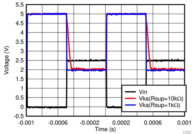
**Figure 9-4. Output Response With Various Cathode Currents**
