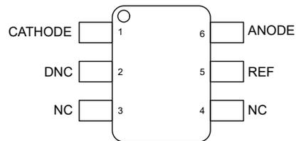
Figure 5-3. DRL Package, 6-Pin SOT-563, TLA431 (Top View)
