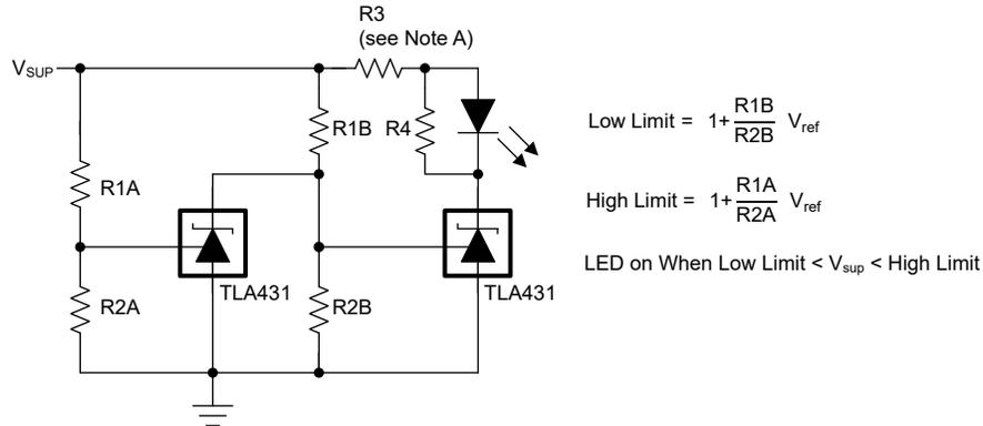
A. Select R3 and R4 to provide the desired LED intensity and cathode current  $\geq 0.2\text{mA}$  to the TLA431 at the available  $V_{SUP}$ .
