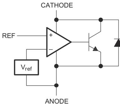
Figure 8-1. Equivalent Schematic
