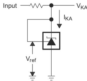
**Figure 7-1. Test Circuit for  $V_{KA} = V_{ref}$**
