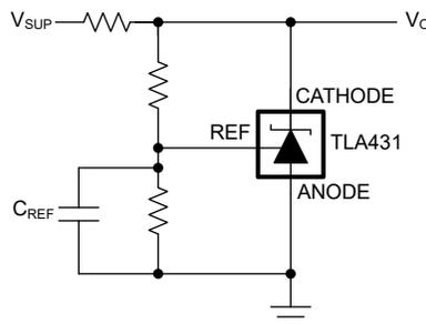
**Figure 8-3. TLA431 with capacitor on REF pin**
