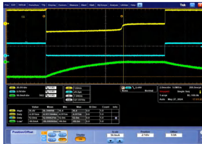
Figure 8-5. CQ Power Up Delay, t_{\text{UVLO}} (Pin mode or the default 00b setting in SPI mode)
