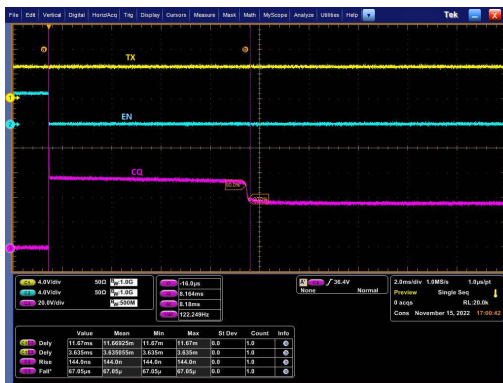
Figure 9-4. CQ in Current Fault Auto Recovery, Low Side Mode
