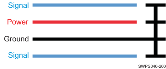
Figure 7-19. Guard Ring Routing
