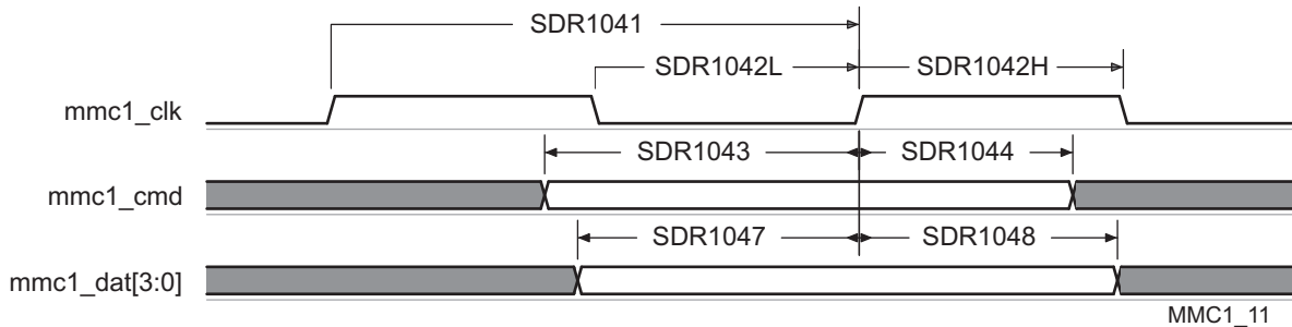
Figure 5-85. MMC/SD/SDIO in - High Speed SDR104 - Receiver Mode
