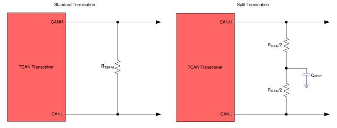
Figure 8-2. CAN Bus Termination Concepts
