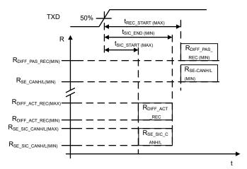
Figure 7-2. TX based Signal Improvement Capability
