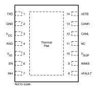
Figure 4-2. DMT Package, 14 Pin (VSON) (Top View)
