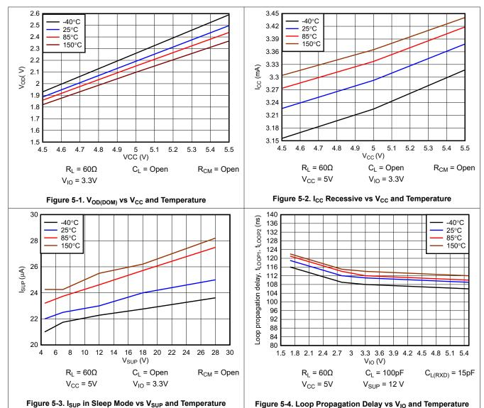
rigure 3-4. Loop Propagation Delay vs vio and Temperature
