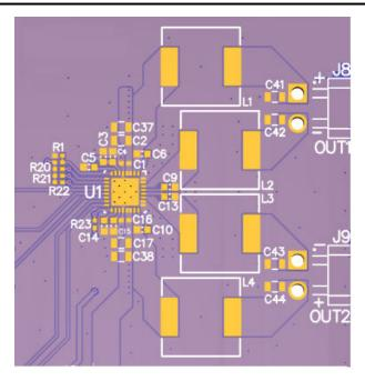
Figure 10-13. 2.0 (Stereo BTL) Top Copper View
