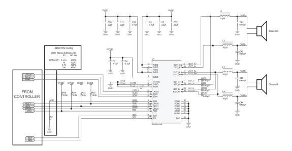
Figure 10-1. 2.0 (Stereo BTL) System Application Schematic
