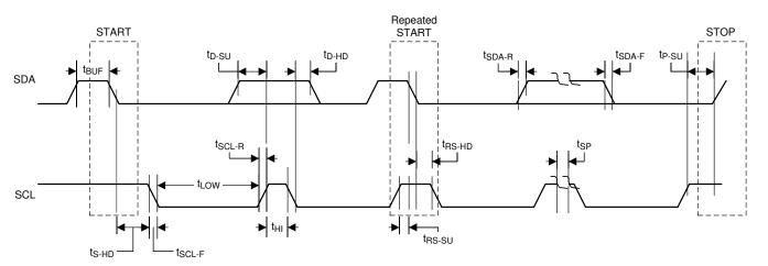
Figure 8-2. I<sup>2</sup>C Communication Port Timing Diagram
