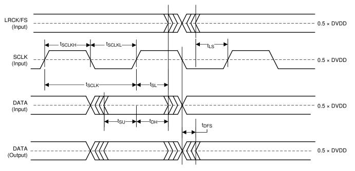
Figure 8-1. Serial Audio Port Timing in Peripheral Mode
