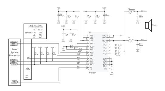
Figure 10-8. Sub-Woofer (PBTL) Application Schematic
