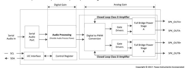
Figure 9-7. Speaker Amplifier Gain
