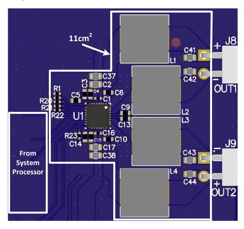
Figure 10-12. 2.0 (Stereo BTL) 3-D View
