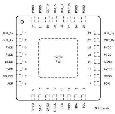
Figure 6-1. RHB Package 32-Pin VQFN
