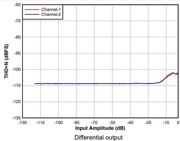
**Figure 5-19. DAC THD+N Level vs Input**
