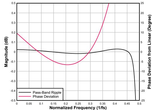
**Figure 6-59. Ultra Low-latency Decimation Filter Pass-Band Ripple and Phase Deviation****Table 6-36. Ultra Low-latency Decimation Filter Specifications**
