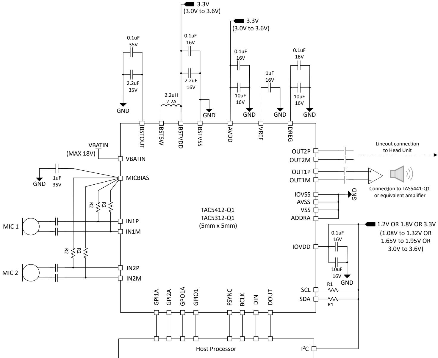
**Figure 8-1. Stereo Microphone with Stereo Lineout Block Diagram**
