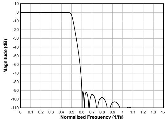
**Figure 6-60. Ultra Low-latency Decimation Filter Magnitude Response**
