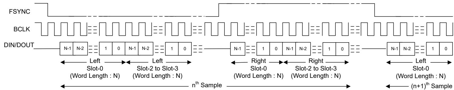
**Figure 6-9. I<sup>2</sup>S Protocol Timing (PASI<sub>\_TX\_OFFSET</sub> = 0 and PASI<sub>\_BCLK\_POL</sub> = 1)**
