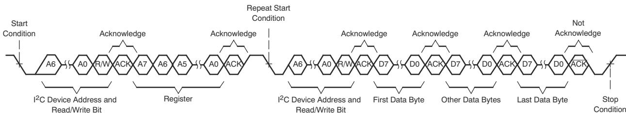
**Figure 6-107. I<sup>2</sup>C Multiple-Byte Read Transfer**
