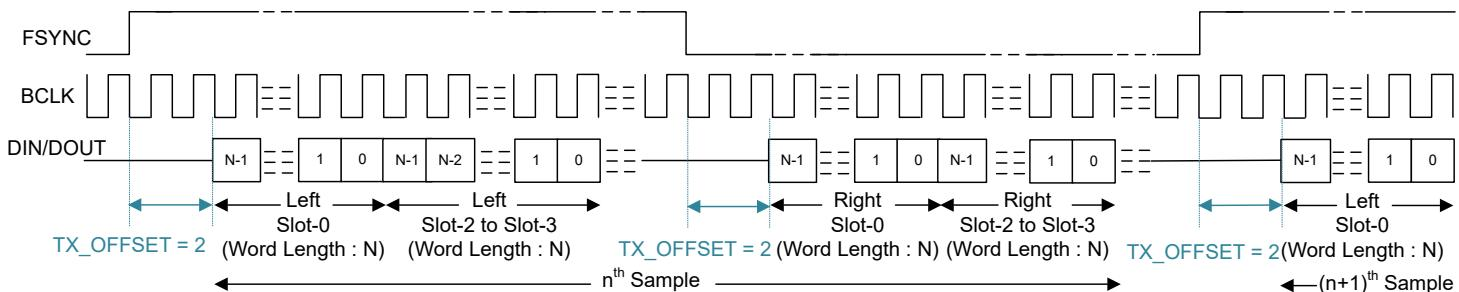
**Figure 6-11. LJ Protocol Timing (TX\_OFFSET = 2)**
