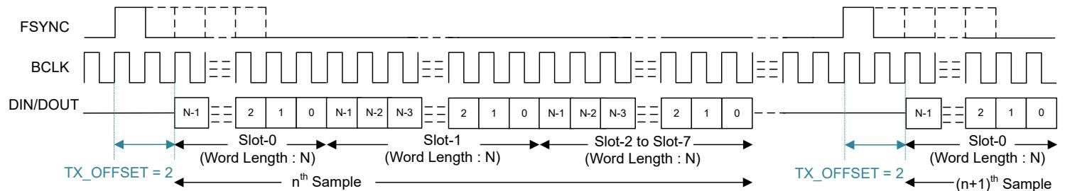
Figure 6-3. TDM Mode Protocol Timing (PASI\_TX\_OFFSET = 2)
