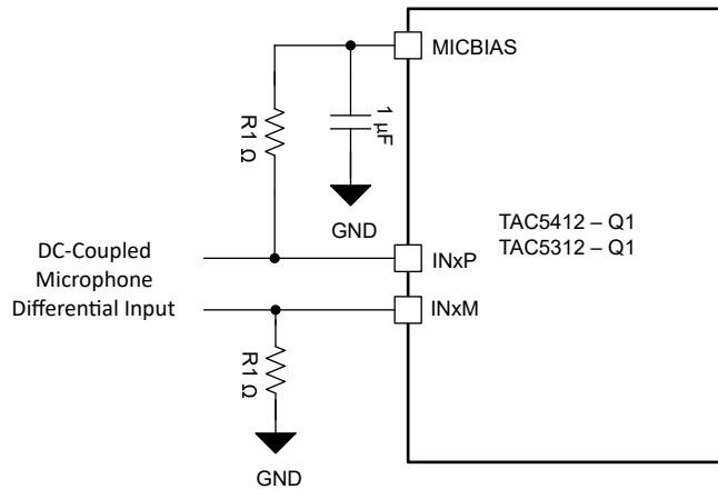
**Figure 6-15. DC-Coupled Microphone or Line Differential Input Connection**
