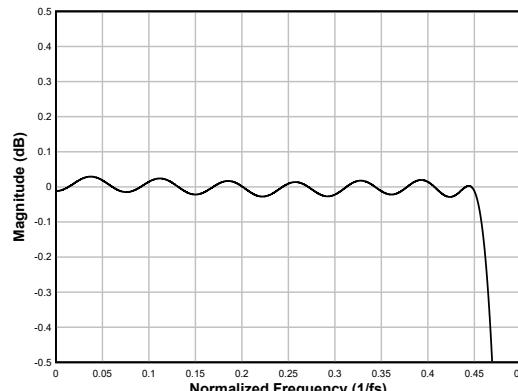
**Figure 6-72. Linear-phase Interpolation Filter Pass-Band Ripple****Table 6-48. Linear-phase Interpolation Filter Specifications**
