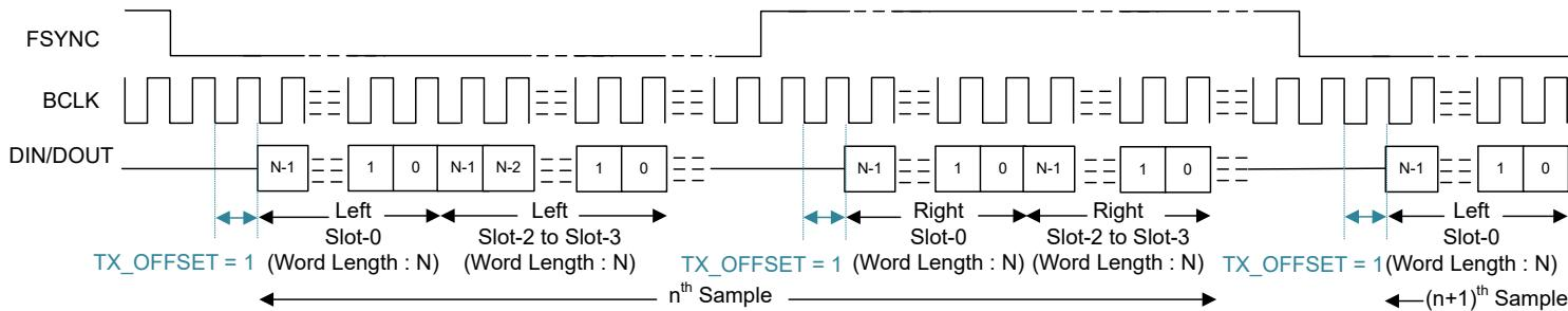
**Figure 6-7. I<sup>2</sup>S Protocol Timing (PASI<sub>\_TX\_OFFSET</sub> = 1)**
