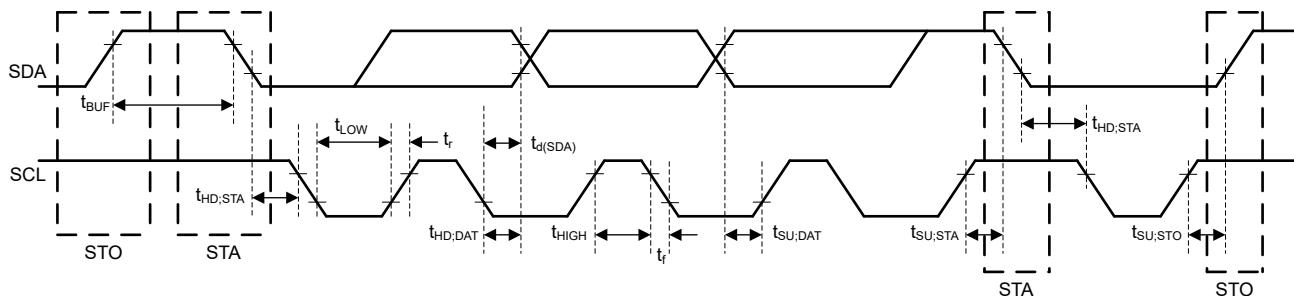
Figure 5-1. I<sup>2</sup>C Interface Timing Diagram
