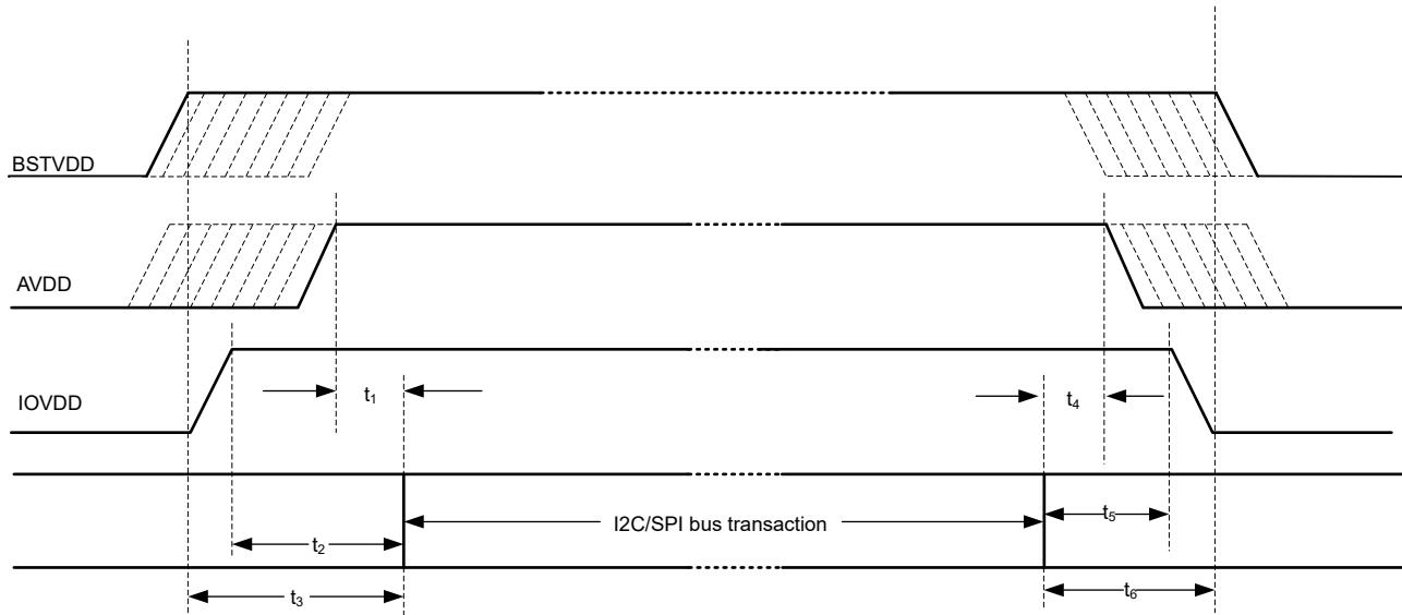
**Figure 8-8. Power-Supply Sequencing Requirement Timing Diagram**
