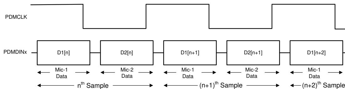
**Figure 6-20. Digital PDM Microphone Protocol Timing Diagram**
