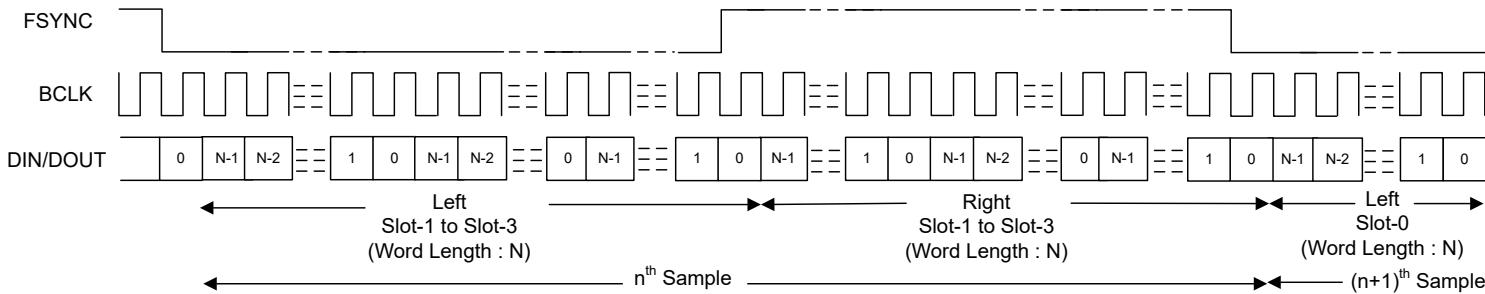
**Figure 6-8. I<sup>2</sup>S Protocol Timing (No Idle BCLK Cycles, PASI<sub>\_TX\_OFFSET</sub> = 0)**
