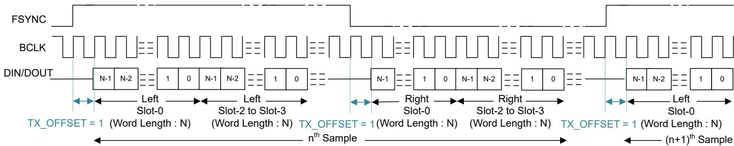
**Figure 6-13. LJ Protocol Timing (TX\_OFFSET = 1 and BCLK\_POL = 1)**
