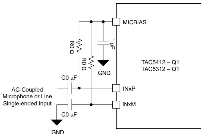
**Figure 6-18. AC-Coupled Microphone or Line Single-Ended Input Connection**
