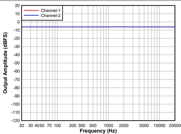
Differential output, -6dBFS input with High-pass filter (HPF)
