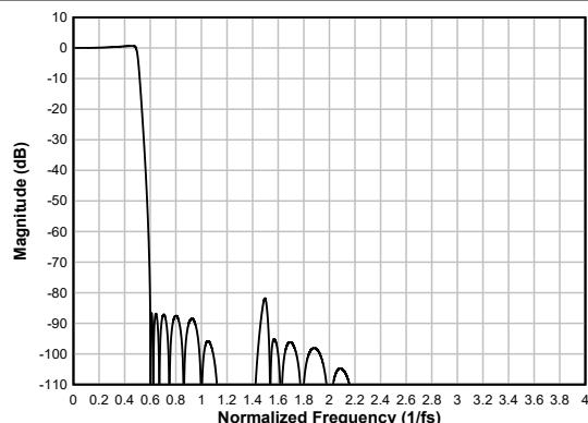
**Figure 6-54. Ultra Low-latency Decimation Filter Magnitude Response**
