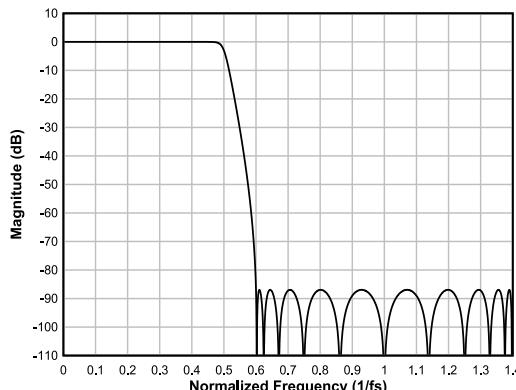
**Figure 6-91. Low-latency Interpolation Filter Magnitude Response**
