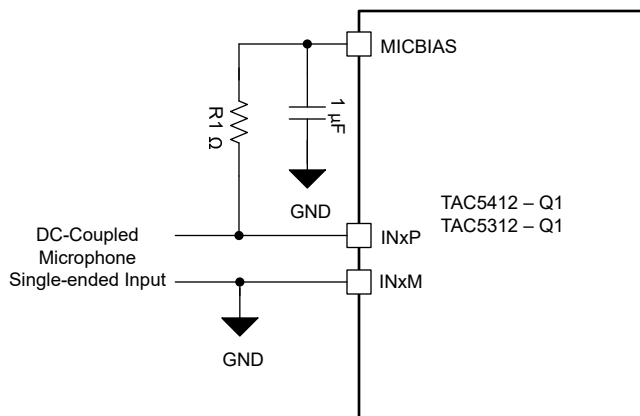
**Figure 6-16. DC-Coupled Microphone or Line Single-Ended Input Connection**
