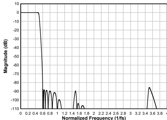
**Figure 6-58. Ultra Low-latency Decimation Filter Magnitude Response**
