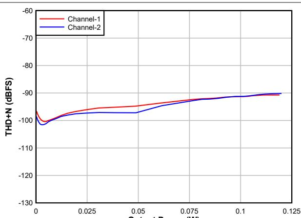
**Figure 5-22. DAC THD+N Level vs Output Power**
