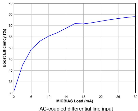
**Figure 5-18. Boost Efficiency vs MICBIAS Load Current**
