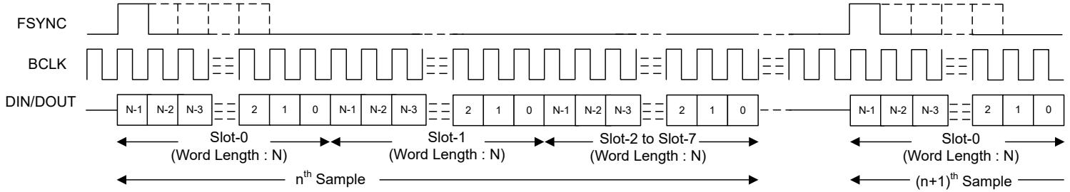
Figure 6-2. TDM Mode Standard Protocol Timing (PASI\_TX\_OFFSET = 0)
