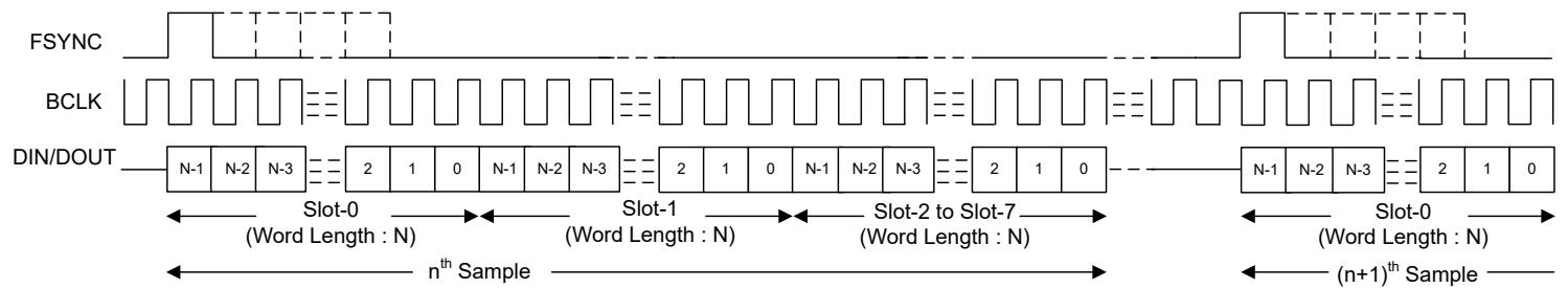
Figure 6-5. TDM Mode Protocol Timing (PASI\_TX\_OFFSET = 0 and PASI\_BCLK\_POL = 1)
