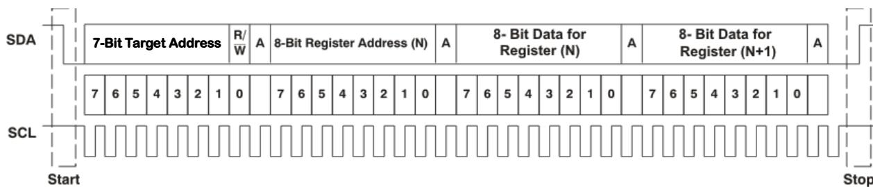
**Figure 6-103. Typical I<sup>2</sup>C Sequence**
