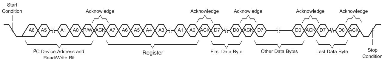
**Figure 6-105. I<sup>2</sup>C Multiple-Byte Write Transfer**
