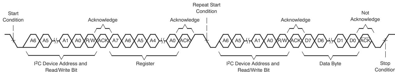
**Figure 6-106. I<sup>2</sup>C Single-Byte Read Transfer**
