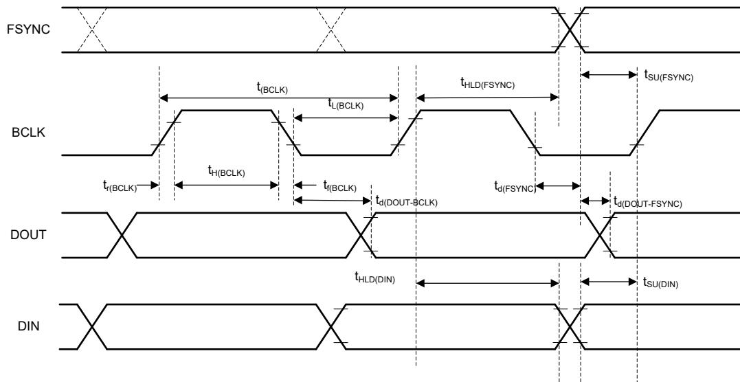
**Figure 5-3. TDM (With BCLK\_POL = 1), I<sup>2</sup>S, and LJ Interface Timing Diagram**
