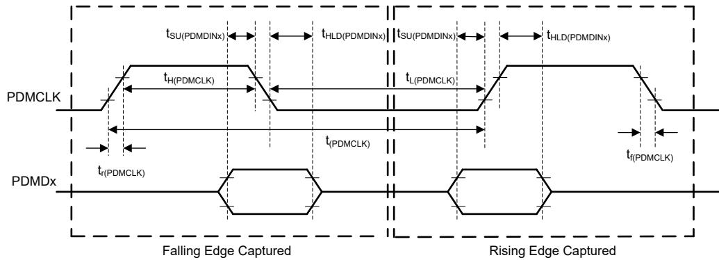
**Figure 5-4. PDM Digital Microphone Interface Timing Diagram**
