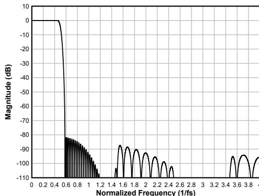
**Figure 6-71. Linear-phase Interpolation Filter Magnitude Response**
