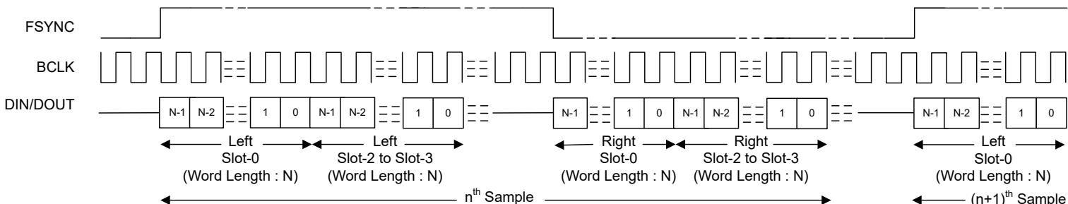
**Figure 6-10. LJ Mode Standard Protocol Timing (TX\_OFFSET = 0)**
