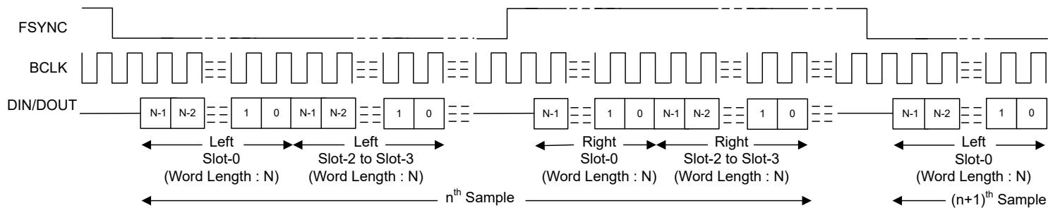
**Figure 6-6. I<sup>2</sup>S Mode Standard Protocol Timing (PASI<sub>\_TX\_OFFSET</sub> = 0)**
