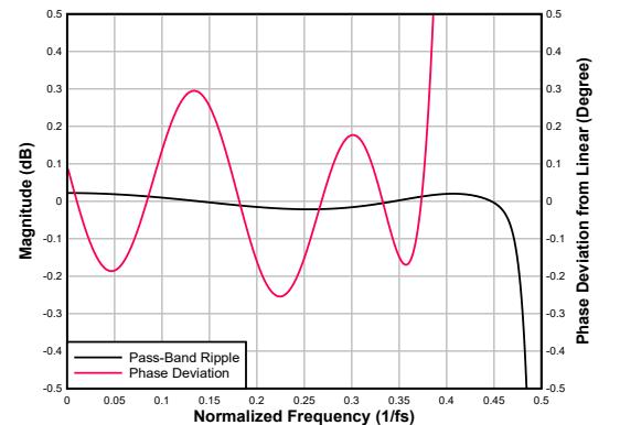
**Figure 6-47. Low-latency Decimation Filter Pass-Band Ripple and Phase Deviation**
