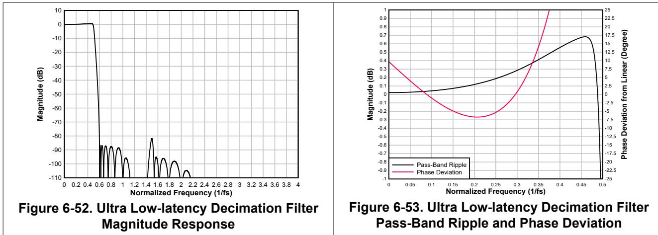
**Figure 6-52. Ultra Low-latency Decimation Filter Magnitude Response**
