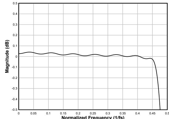
**Figure 6-27. Linear-phase Decimation Filter Pass-Band Ripple**
