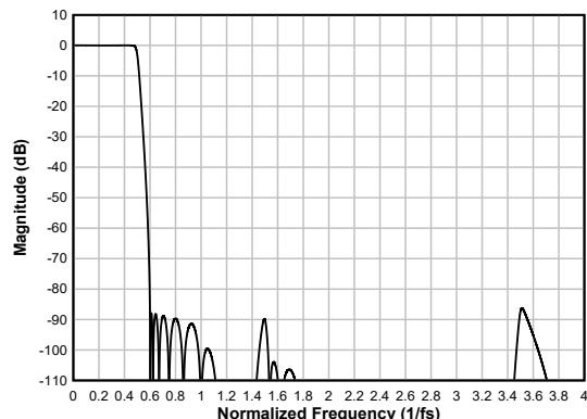
**Figure 6-56. Ultra Low-latency Decimation Filter Magnitude Response**
