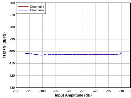
DC-coupled differential line input, with DC common-mode
