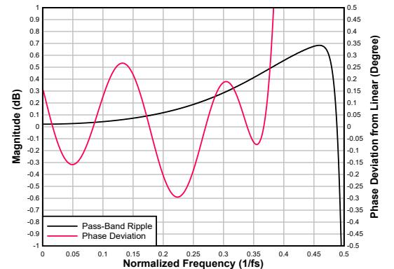
**Figure 6-45. Low-latency Decimation Filter Pass-Band Ripple and Phase Deviation**
