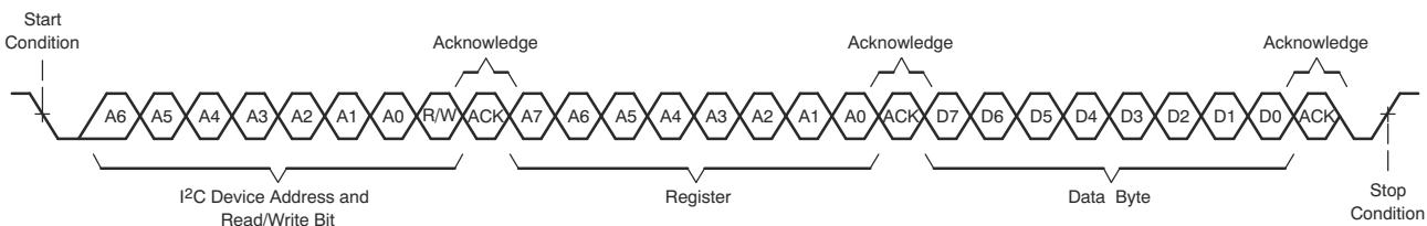
**Figure 6-104. I<sup>2</sup>C Single-Byte Write Transfer**
