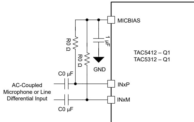
**Figure 6-17. AC-Coupled Microphone or Line Differential Input Connection**
