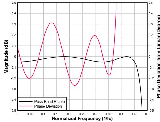
**Figure 6-90. Low-latency Interpolation Filter Pass-Band Ripple and Phase Deviation****Table 6-57. Low-latency Interpolation Filter Specifications**
