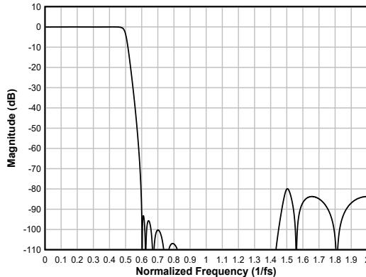
**Figure 6-89. Low-latency Interpolation Filter Magnitude Response**
