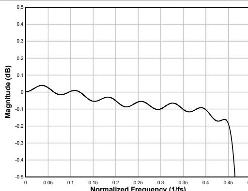
**Figure 6-76. Linear-phase Interpolation Filter Pass-Band Ripple**
