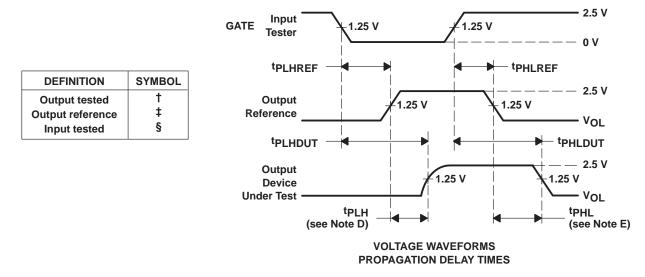
NOTES: A. All input pulses are supplied by generators having the following characteristics: PRR  $\leq$  10 MHz,  $Z_O = 50 \ \Omega$ ,  $t_f \leq 2 \ ns$ .
