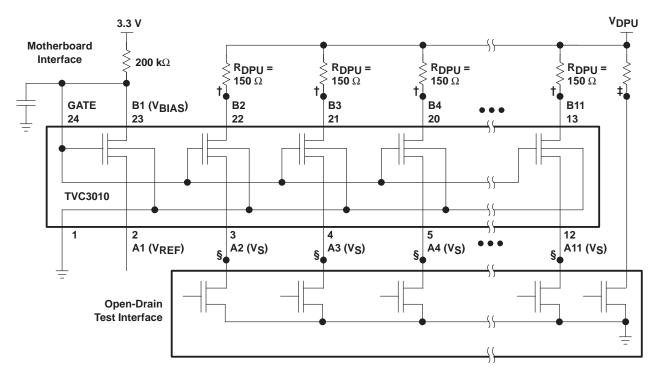
TESTER CALIBRATION SETUP (see Note C)
