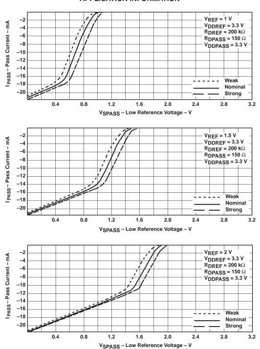
Figure 5. Electrical Characteristics at Low V<sub>REF</sub> Voltages
