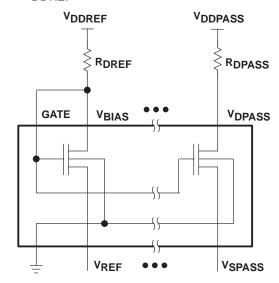
Figure 4. TI SPICE Simulation Schematic and Voltage-Node Names
