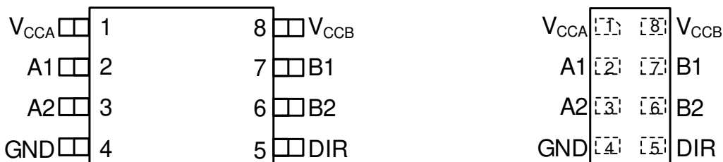
Figure 5-1. DCU and DTT Package, 8-Pin VSSOP and SON Transparent (Top View)
