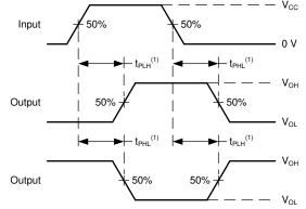
(1) The greater between t<sub>PLH</sub> and t<sub>PHL</sub> is the same as t<sub>pd</sub>. Figure 6-2. Voltage Waveforms Propagation Delays
