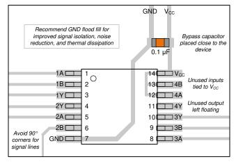
Figure 8-3. Example Layout for the SN74LVC7266A-Q1
