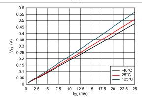
Figure 5-3. Output Voltage vs Current in LOW State; 3.3V
