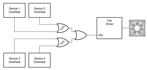
Figure 8-1. Typical Application Block Diagram
