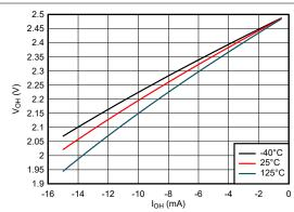
Figure 5-4. Output Voltage vs Current in HIGH State; 2.5V Supply
