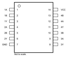
Figure 4-1. SN74LVC7032A-Q1 BQA Package, 14-Pin WQFN (Top View)
