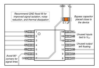
Figure 8-3. Example Layout for the SN74LVC7032A-Q1
