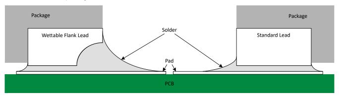
Figure 7-2. Simplified Cutaway View of Wettable-Flank QFN Package and Standard QFN Package After Soldering
