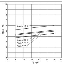
Figure 5-7. Typical Propagation Delay of High-to-Low (B to A) vs | Figure 5-8. Typical Propagation Delay of Low-to-High (B to A) vs Load Capacitance  $T_A = 25$ °C,  $V_{CCA} = 2.5V$
