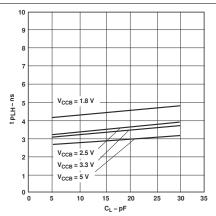
Figure 5-12. Typical Propagation Delay of Low-to-High (B to A) vs Load Capacitance T<sub>A</sub> = 25°C, V<sub>CCA</sub> = 3.3V
