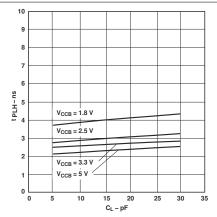
Figure 5-16. Typical Propagation Delay of Low-to-High (B to A) vs Load Capacitance  $T_A = 25^{\circ}C$ ,  $V_{CCA} = 5V$
