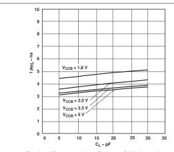
Load Capacitance  $T_A = 25$ °C,  $V_{CCA} = 2.5V$
