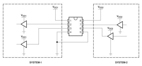
Figure 8-1. Unidirectional Logic Level-Shifting Application
