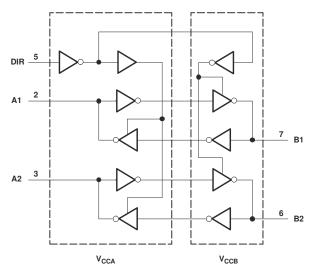
Figure 7-1. Logic Diagram (Positive Logic)
