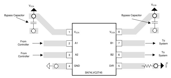
Figure 8-3. SN74LVC2T45 Layout Example
