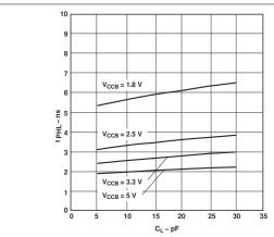
Figure 5-13. Typical Propagation Delay of High-to-Low (A to B) vs Load Capacitance  $T_A = 25^{\circ}C$ ,  $V_{CCA} = 5V$
