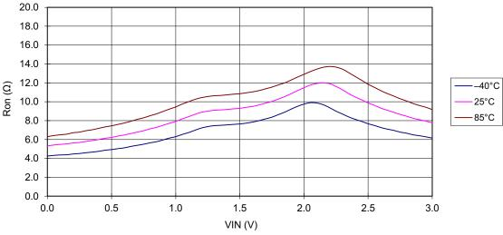
Pin: A-B,  $V_{CC}$  = 3 V,  $I_S$  = 24 mA
