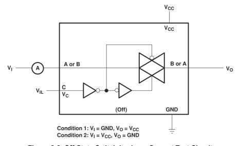
Figure 8-2. Off-State Switch Leakage-Current Test Circuit
