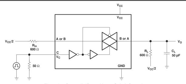
Figure 8-7. Crosstalk (Control Input, Switch Output)
