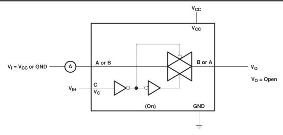
Figure 8-3. On-State Leakage-Current Test Circuit
