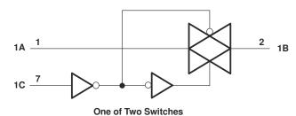
Logic Diagram, Each Switch (Positive Logic)
