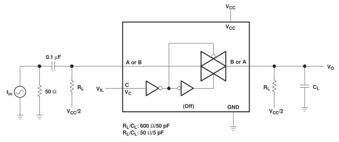
Figure 8-8. Feedthrough (Switch Off)
