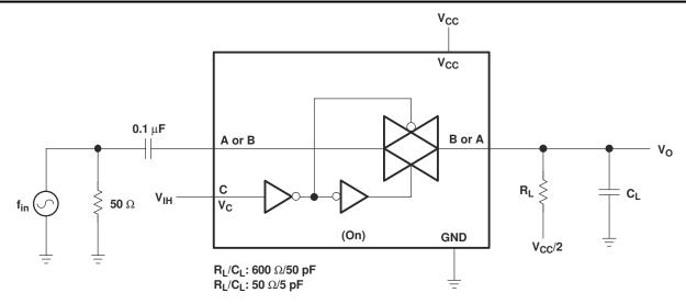
Figure 8-5. Frequency Response (Switch On)
