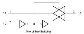
Figure 9-1. Logic Diagram, Each Switch (Positive Logic)
