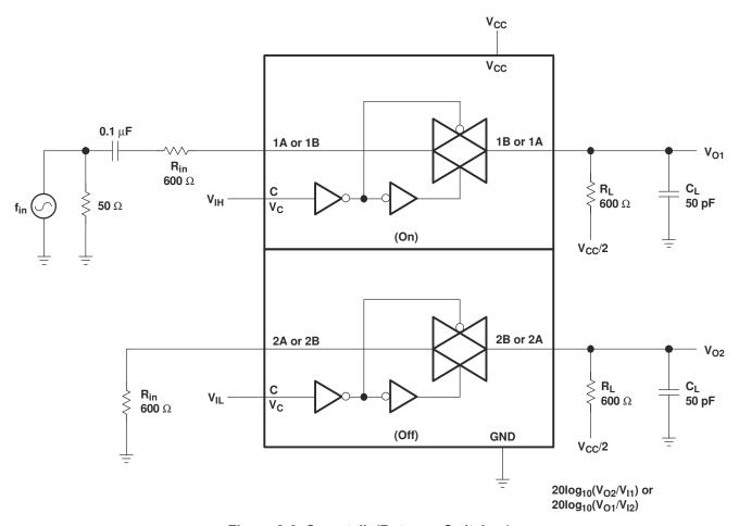
Figure 8-6. Crosstalk (Between Switches)
