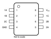
Figure 6-1. DCU Package 8-Pin VSSOP Top View
