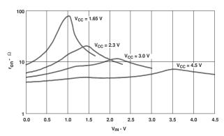
Figure 7-1. Typical  $r_{on}$  as a Function of Input Voltage (V<sub>I</sub>) for  $V_{I}$  = 0 to  $V_{CC}$
