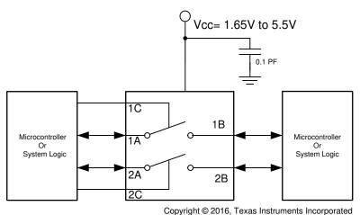
Figure 10-1. Typical Application Schematic
