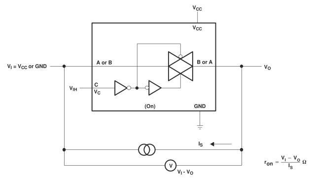
Figure 8-1. On-State Resistance Test Circuit
