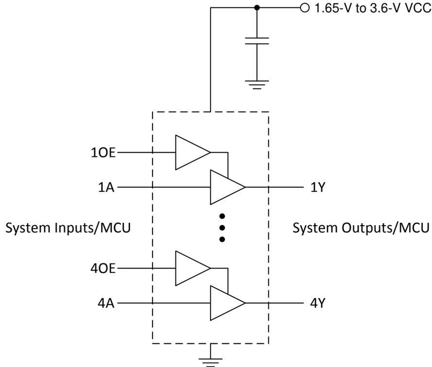
**Figure 8-1. Typical Buffer Application and Supply Voltage**
