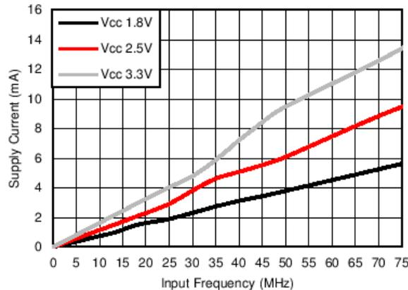
Figure 8-2. Supply Current vs Input Frequency
