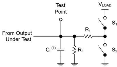
(1) C<sub>L</sub> includes probe and test-fixture capacitance.
