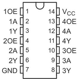
**Figure 4-1. SN74LVC126A D, DB, DGV, NS, or PW Package; 14-Pin SOIC, SSOP, TVSOP, SOP or TSSOP (Top View)**
