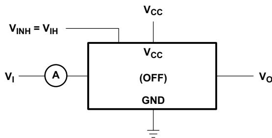
Condition 1:  $V_I = 0, V_O = V_{CC}$
