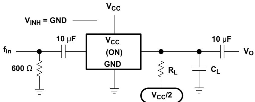
Figure 6-9. Sine-Wave Distortion
