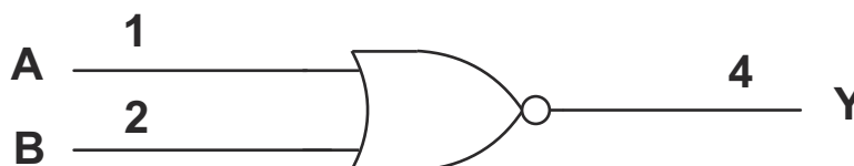
Simplified Logic Diagram (Positive Logic)
