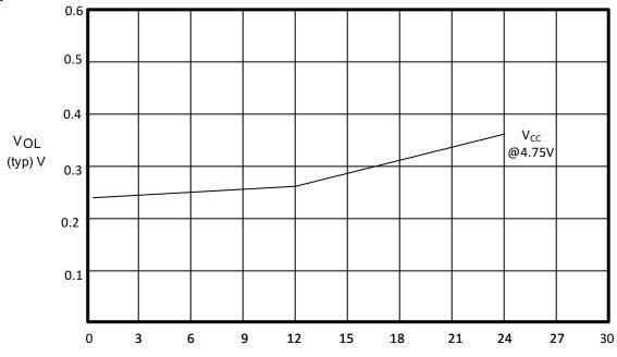
$I_{OL}$  (mA) Figure 3.  $V_{OL}$  vs  $I_{OL}$
