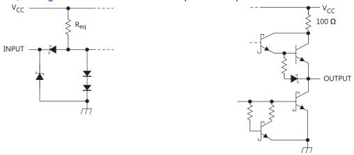
Figure 7. Equivalent of Each Input
