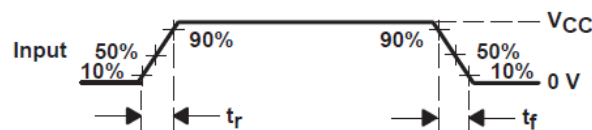
Figure 6-4. Voltage Waveform Input Rise and Fall Times
