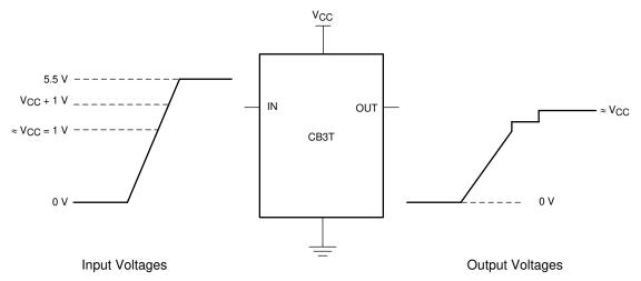
If the input high voltage ( $V_{IH}$ ) level is greater than or equal to  $V_{CC}$  + 1V, and less than or equal to 5.5V, the output high voltage ( $V_{OH}$ ) level is equal to approximately the  $V_{CC}$  voltage level.
