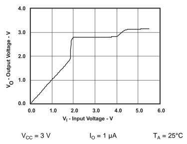
Figure 10. Data Output Voltage vs Data Input Voltage
