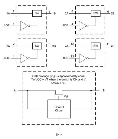
Figure 7. Simplified Schematic, Each FET Switch (SW)
