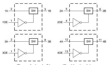
Figure 8. Logic Diagram (Positive Logic)
