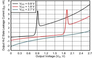
Figure 6-3. Output High-Impedance State Leakage Current Across Output Voltage, 0.8-, 1.8-, and 2.7-V Supply
