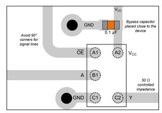
Figure 11-2. Example Layout for YZP Package
