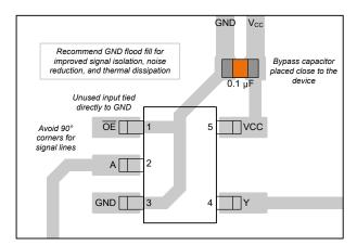
Figure 11-1. Example Layout for DCK Package
