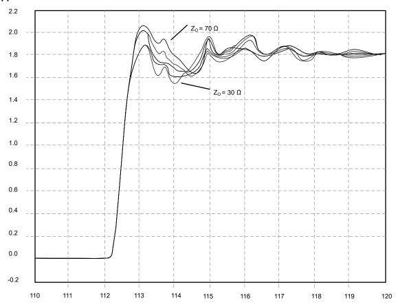
Figure 9-2. Simulated Output Voltage Waveforms for AUC Family Directly Driving Short (< 15 cm) Transmission Lines With Characteristic Impedances from 30 to 70  $\Omega$  (Volts vs Nanoseconds)
