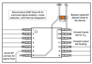
Figure 8-3. Example Layout for the SN74AHCT32-Q1
