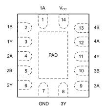
Figure 4-2. BQA (Preview) Package, 14-Pin WQFN (Top View)
