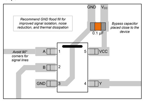
Figure 8-3. Example Layout for the SN74AHCT1G14
