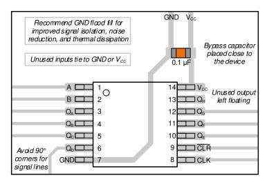
Figure 8-3. Example Layout for the SN74AHCT164-Q1
