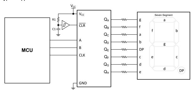
Figure 8-1. Typical Application Block Diagram
