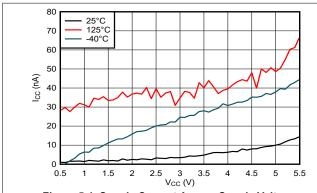
Figure 5-1. Supply Current Across Supply Voltage
