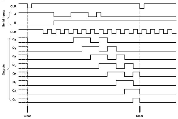
Figure 8-2. Application Timing Diagram
