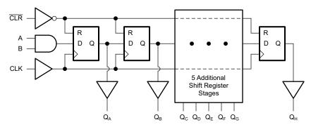
Figure 7-1. Logic Diagram (Positive Logic) for SN74AHCT164-Q1
