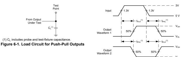
(1) The greater between  $t_{\text{PLH}}$  and  $t_{\text{PHL}}$  is the same as  $t_{\text{pd}}.$
