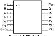
Figure 4-1. PW Package, 14-Pin TSSOP (Top View)
