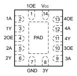
Figure 5-2. BQA Package, WQFN 14-Pin (Transparent Top View)
