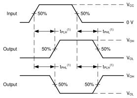
(1) The greater between  $t_{\text{PLH}}$  and  $t_{\text{PHL}}$  is the same as  $t_{\text{pd}}.$
