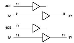
Logic Diagram (Positive Logic)
