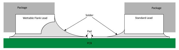
Figure 8-1. Simplified Cutaway View of Wettable-Flank QFN Package and Standard QFN Package After Soldering
