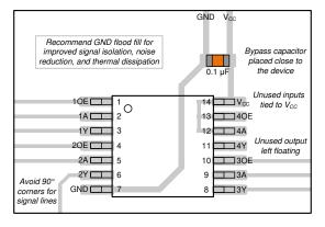
Figure 9-3. Example Layout for the SN74AHC126-Q1
