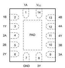
Figure 3-2. BQA Package, 14-Pin WQFN (Top View)
