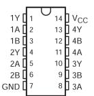
Figure 4-1. PW Package (Top View)
