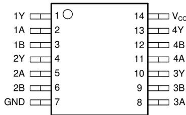
**Figure 3-1. SN54AHC02 J or W Package, 14-Pin (Top View)**
