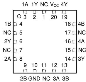
**Figure 3-3. SN54AHC02 FK Package, 20-Pin (Top View)**
