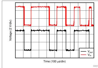
Figure 8-2. Waveform for Non-Debounced Switch
