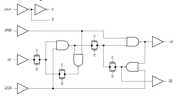
Figure 7-1. Logic Diagram (Positive Logic) for one channel of SN74ACT74-Q1
