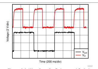
Figure 8-3. Waveform for Debounced Switch
