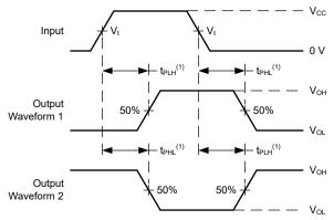
(1) The greater between  $t_{\text{PLH}}$  and  $t_{\text{PHL}}$  is the same as  $t_{\text{pd}}$ .
