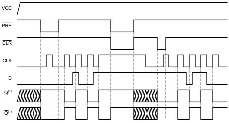
(1) Crosshatch indicates unknown output state. Unknown outputs are either high or low. Q and  $\overline{Q}$  are in opposite states when unknown.
