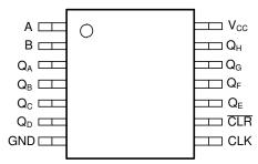
Figure 4-1. PW Package, 14-Pin TSSOP (Top View)
