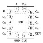
Figure 4-2. WBQA Package 14-Pin WQFN (Top View)
