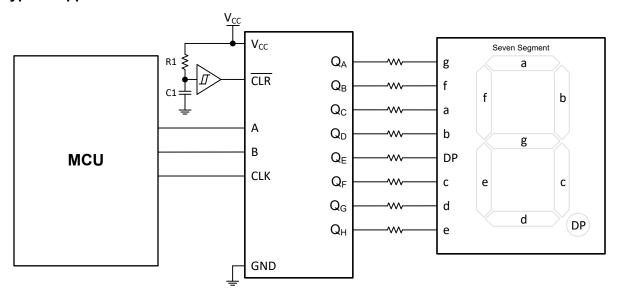
Figure 8-1. Typical Application Block Diagram
