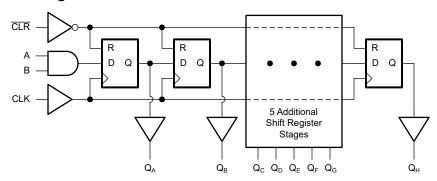
Figure 7-1. Logic Diagram (Positive Logic) for SN74ACT164-Q1
