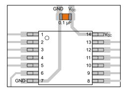
Figure 8-4. Example Bypass Capacitor Placement for TSSOP and Similar Packages
