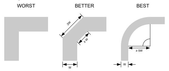
Figure 8-3. Example Trace Corners for Improved Signal Integrity
