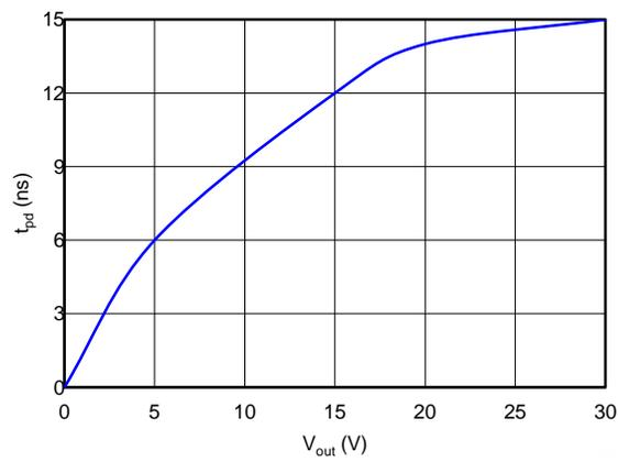
**Figure 1. Time Low to High vs  $V_{OUT}$**
