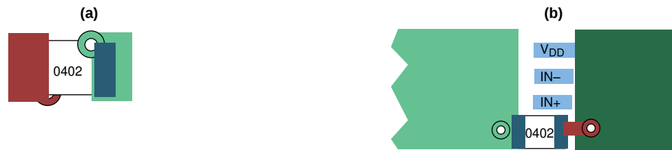
Figure 28. Typical Decoupling Capacitor Layouts
