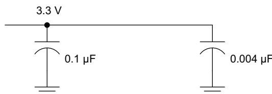
Figure 9-2. Recommended M-LVDS Bypass Capacitor Layout
