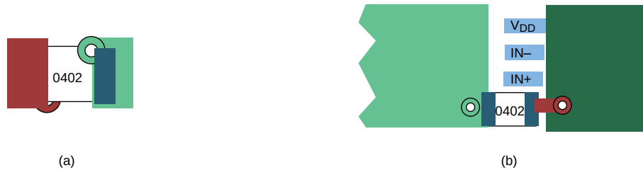
Figure 33. Typical Decoupling Capacitor Layouts
