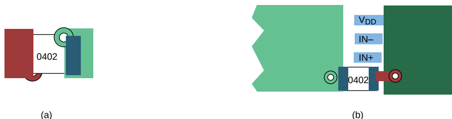
Figure 48. Typical Decoupling Capacitor Layouts
