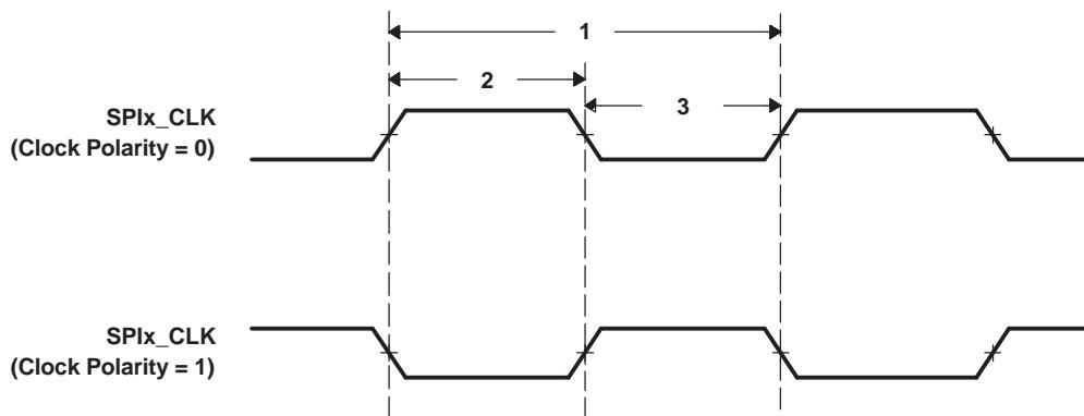
**Figure 6-62. SPI\_CLK Timing**
