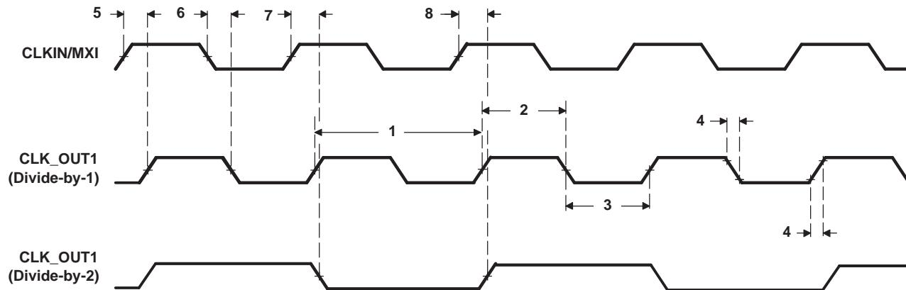
**Figure 6-17. CLK\_OUT1 Timing**
