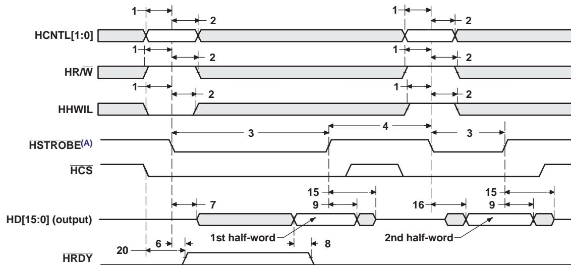
A.  $\overline{\text{HSTROBE}}$  refers to the following logical operation on  $\overline{\text{HCS}}$ ,  $\overline{\text{HDS1}}$ , and  $\overline{\text{HDS2}}$ : [NOT(HDS1 XOR HDS2)] OR HCS.
