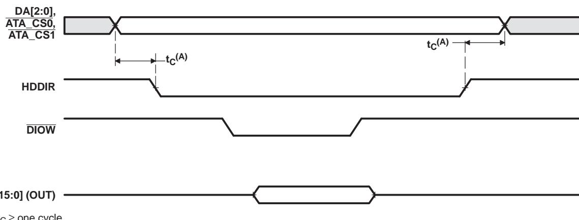
**Figure 6-38. ATA/CF HDDIR Taskfile Write/Single PIO Write Timing**
