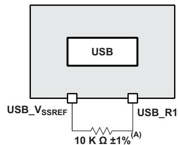
A. Place the  $10\text{ K}\Omega \pm 1\%$  as close to the device as possible.
