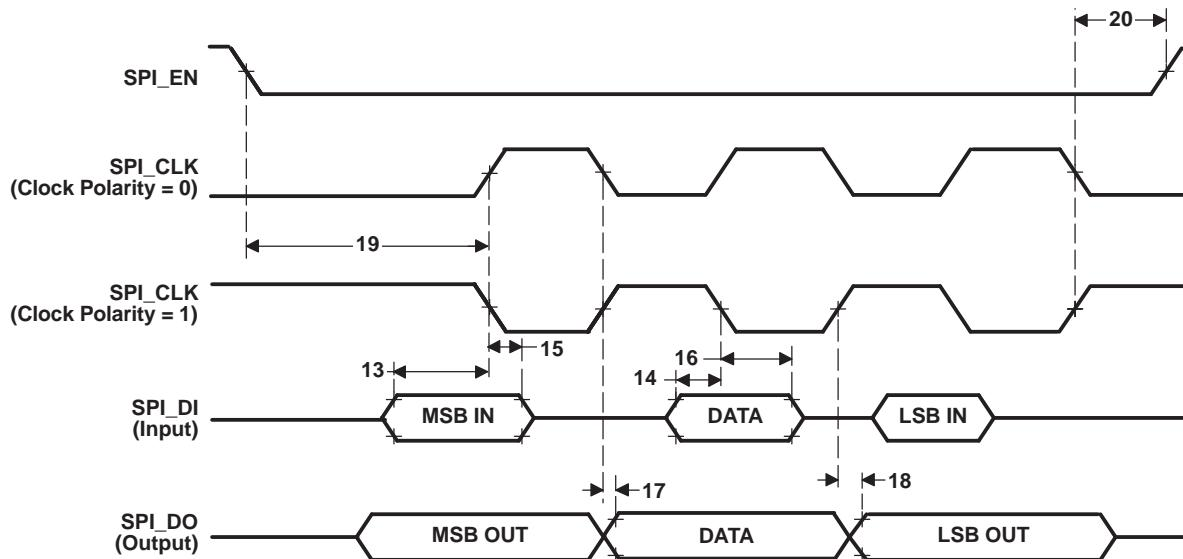
**Figure 6-64. SPI Master Mode External Timing (Clock Phase = 1)**
