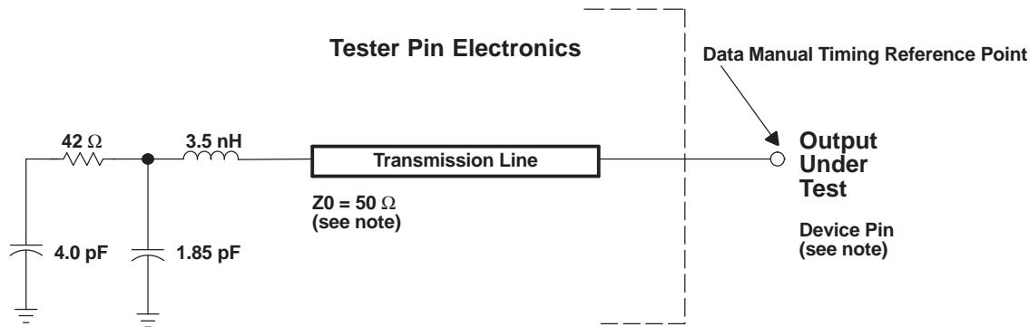
NOTE: The data manual provides timing at the device pin. For output timing analysis, the tester pin electronics and its transmission line effects must be taken into account. A transmission line with a delay of 2 ns or longer can be used to produce the desired transmission line effect. The transmission line is intended as a load only. It is not necessary to add or subtract the transmission line delay (2 ns or longer) from the data manual timings.
