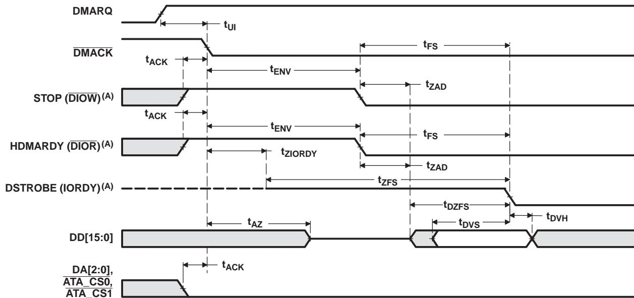
A. The definitions for the DIOW:STOP, DIOR:HDMARDY, and IORDY:DSTROBE signal lines are not in effect until DMARQ and DMACK are asserted.
