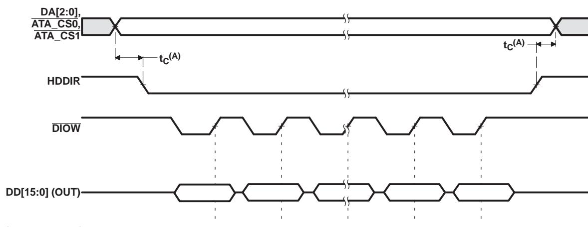
**Figure 6-39. ATA/CF HDDIR PIO Postwrite Start Timing**
