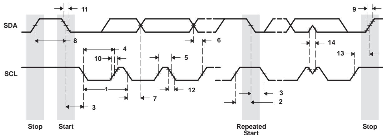
**Figure 6-65. I<sup>2</sup>C Receive Timings**
