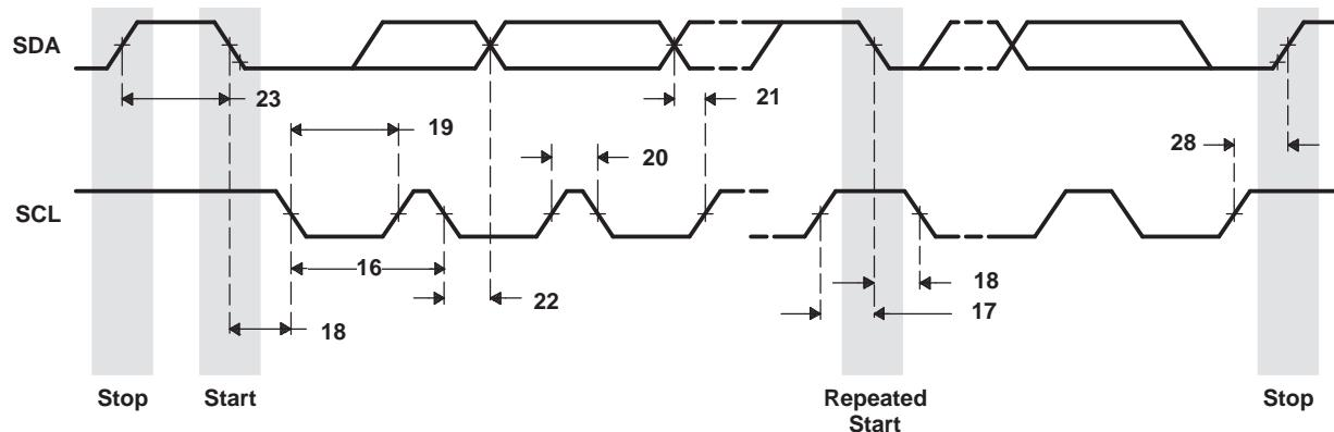
**Figure 6-66. I<sub>2</sub>C Transmit Timings**
