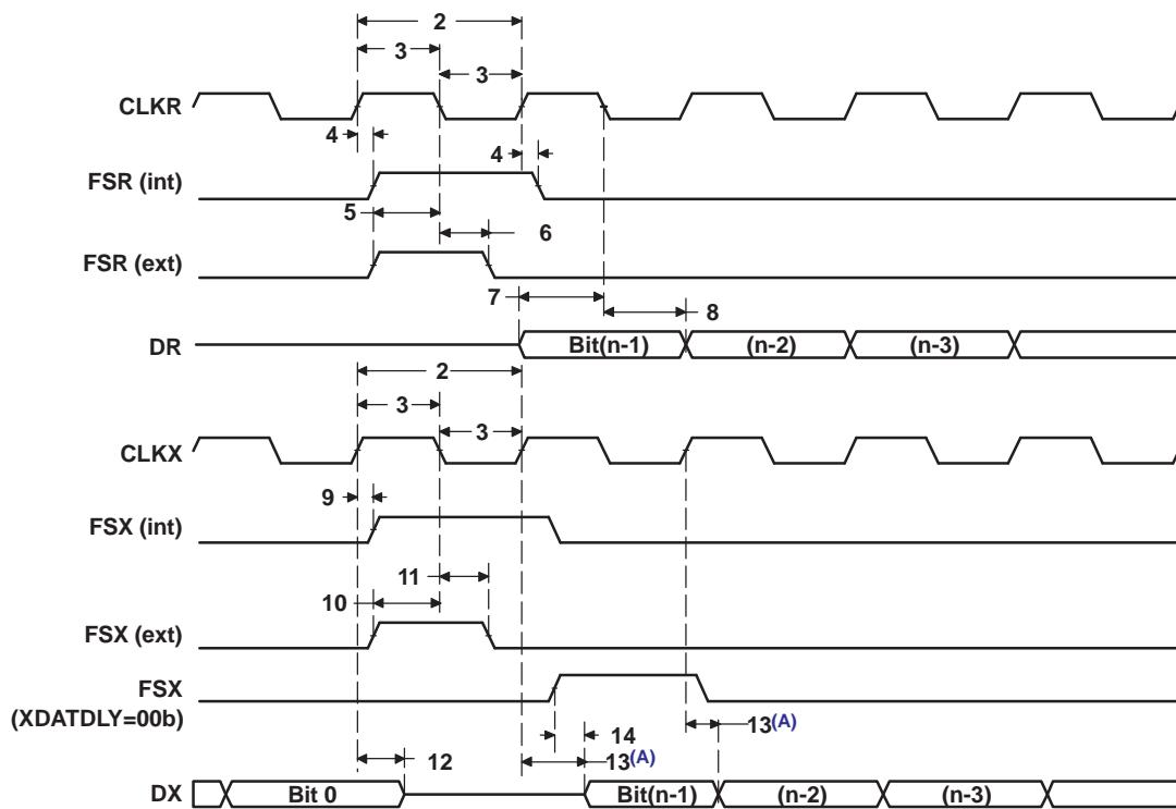
A. Parameter No. 13 applies to the first data bit *only* when XDATDLY ≠ 0.
