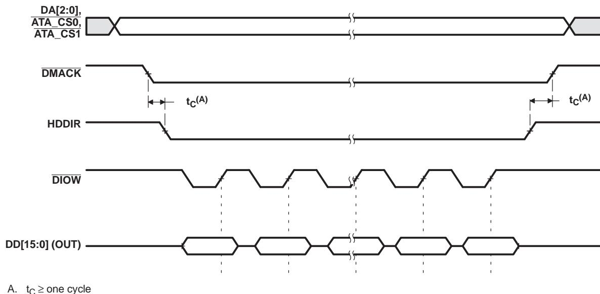
**Figure 6-40. ATA/CF HDDIR Multiword DMA Write Transfer Timing**
