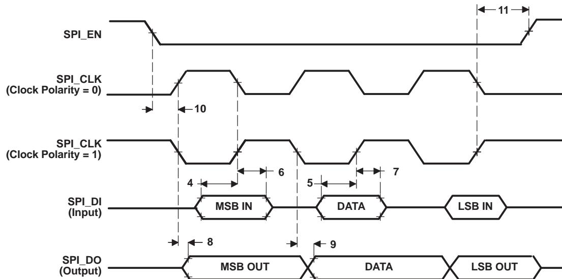
**Figure 6-63. SPI Master Mode External Timing (Clock Phase = 0)**
