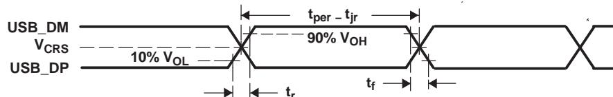
**Figure 6-59. USB2.0 Integrated Transceiver Interface Timing**
