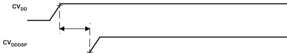
**Figure 6-4. DSP Host-Boot Mode Core Supply Timings**
