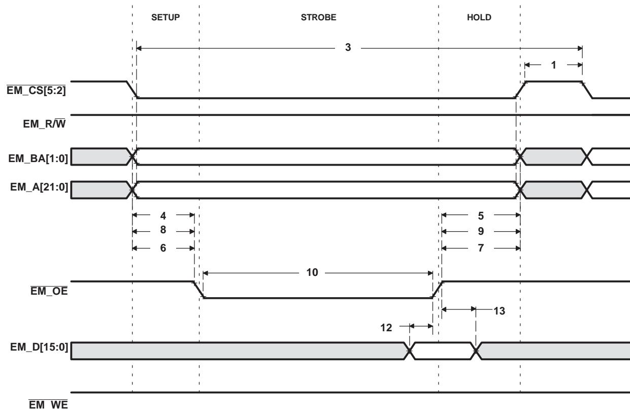
**Figure 6-21. Asynchronous Memory Read Timing for EMIF**
