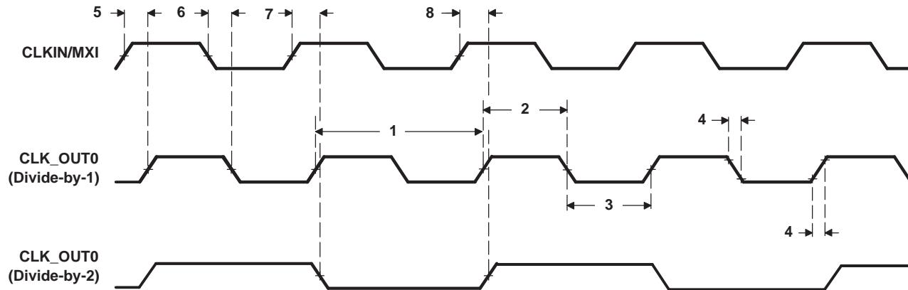
**Figure 6-16. CLK\_OUT0 Timing**
