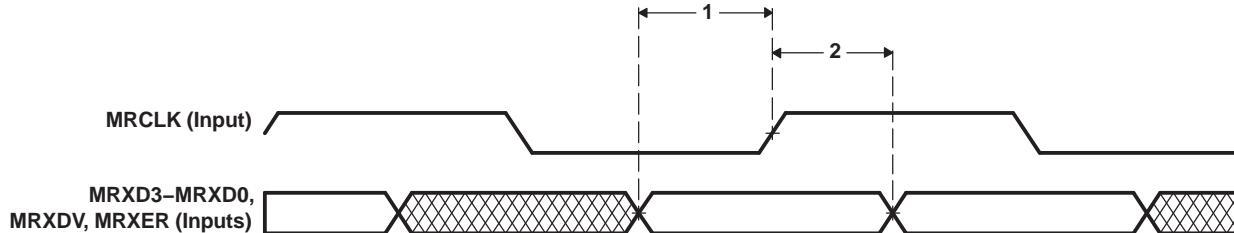
**Figure 6-70. EMAC Receive Interface Timing**
