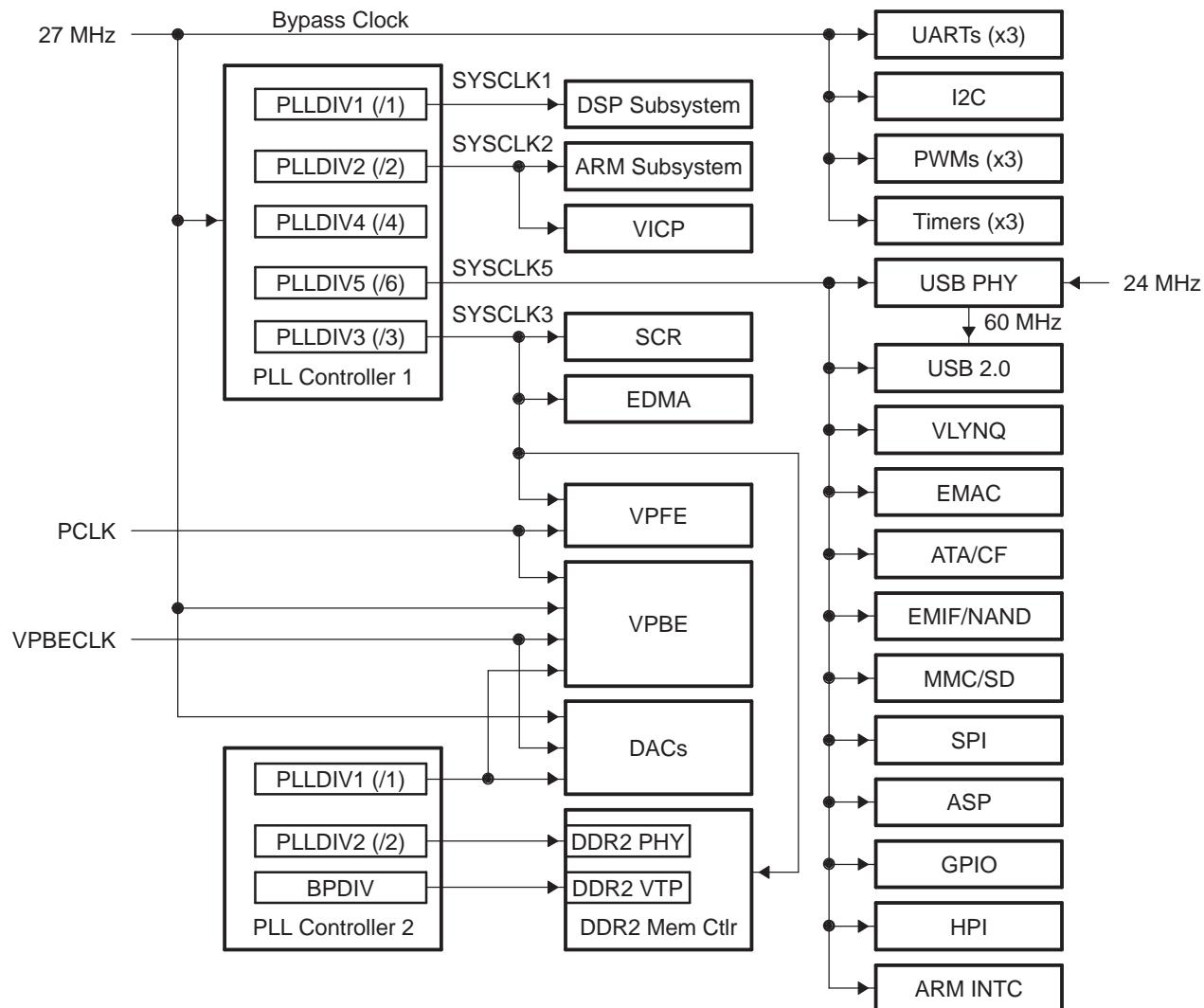
**Figure 6-6. PLL1 and PLL2 Clock Domain Block Diagram**
