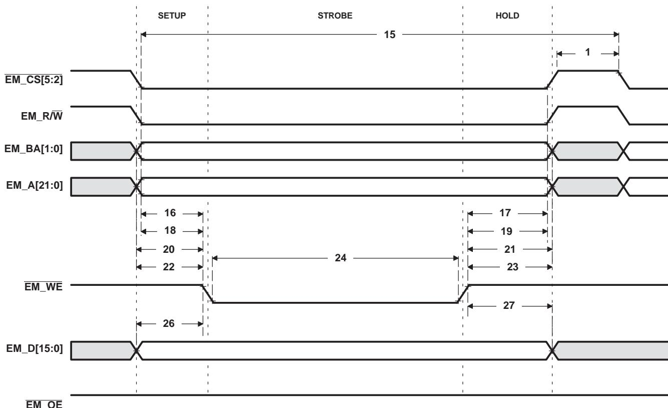
**Figure 6-22. Asynchronous Memory Write Timing for EMIF**
