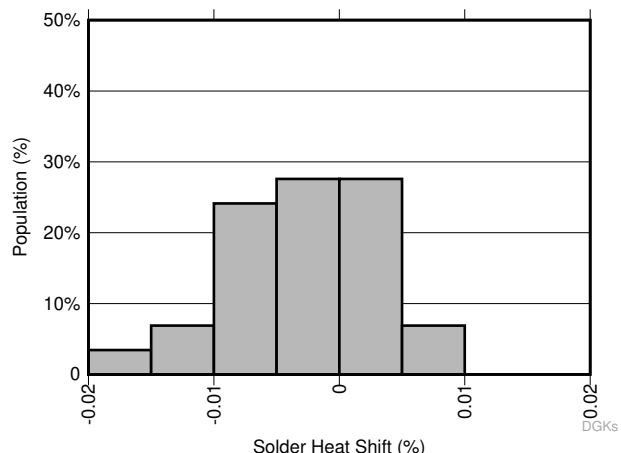
Figure 8-20. Thermal Hysteresis Distribution (Cycle 2) - DGK Package
