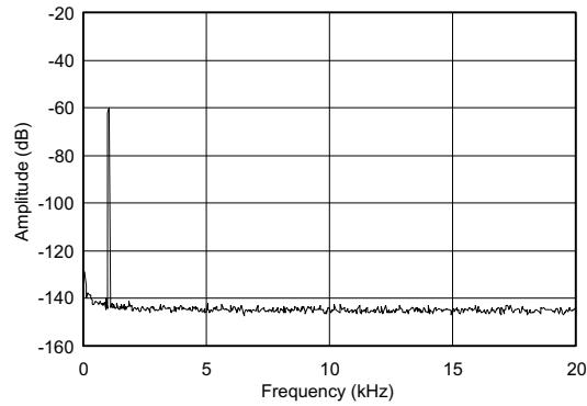
Figure 6. PCM5122 FFT Plot Using a 1-kHz Tone
