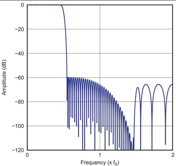
**Figure 22. Normal x4 Interpolation Filter Frequency Response**
