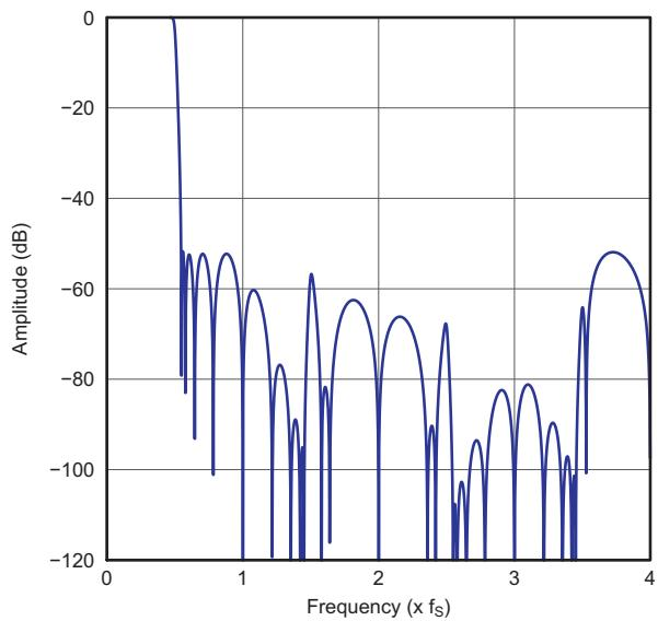
**Figure 28. Low Latency x8 Interpolation Filter Frequency Response**
