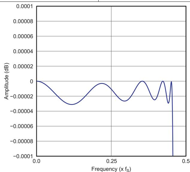
**Figure 36. Low Latency  $\times 2$  Interpolation Filter Passband Ripple**
