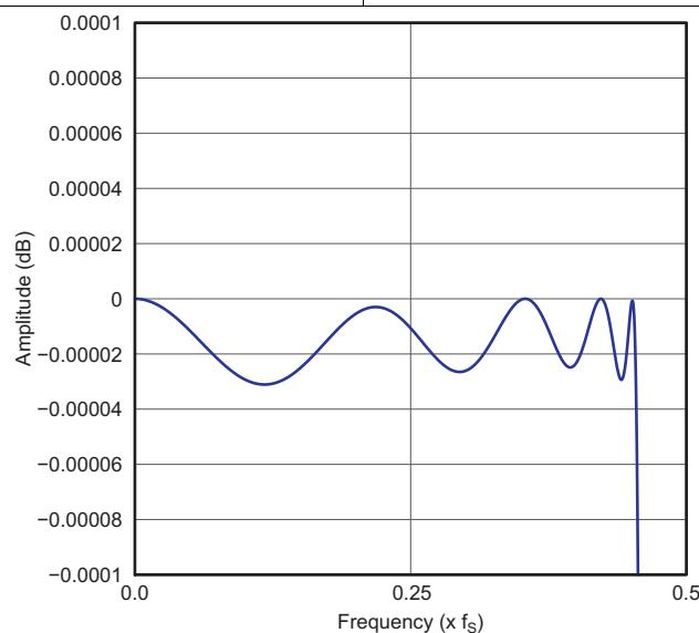
**Figure 33. Low Latency x4 Interpolation Filter Passband Ripple**
