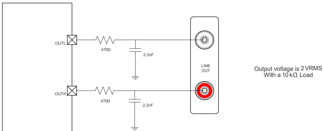
**Figure 61. Recommended Output Lowpass Filter for 10-k $\Omega$  Operation**
