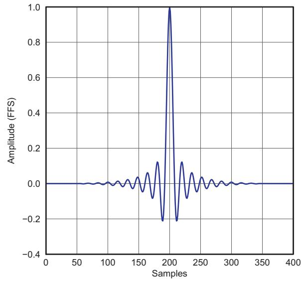
**Figure 20. Normal x8 Interpolation Filter Impulse Response**
