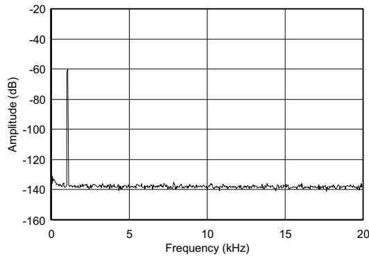
Figure 5. PCM5121 FFT Plot Using a 1-kHz Tone
