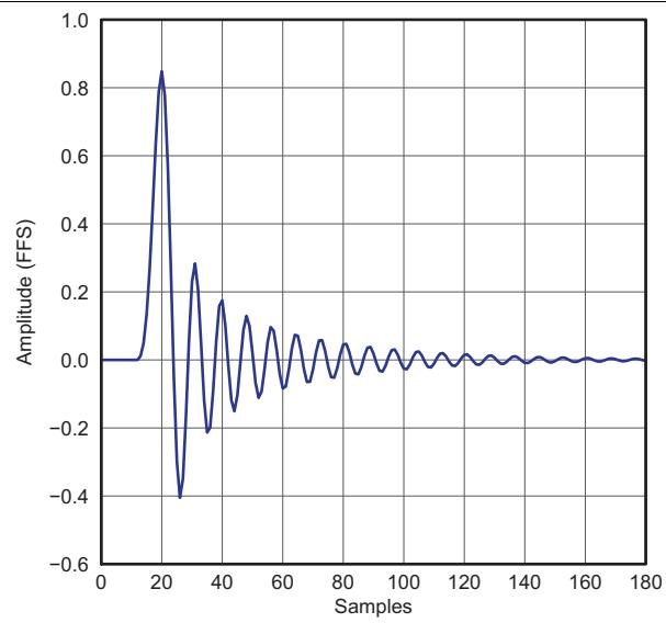
**Figure 32. Low Latency x4 Interpolation Filter Impulse Response**
