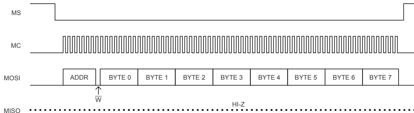
**Figure 68. Serial Control Format; Write, Multiple Byte**
