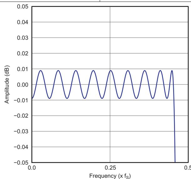
**Figure 27. Normal x2 Interpolation Filter Passband Ripple**
