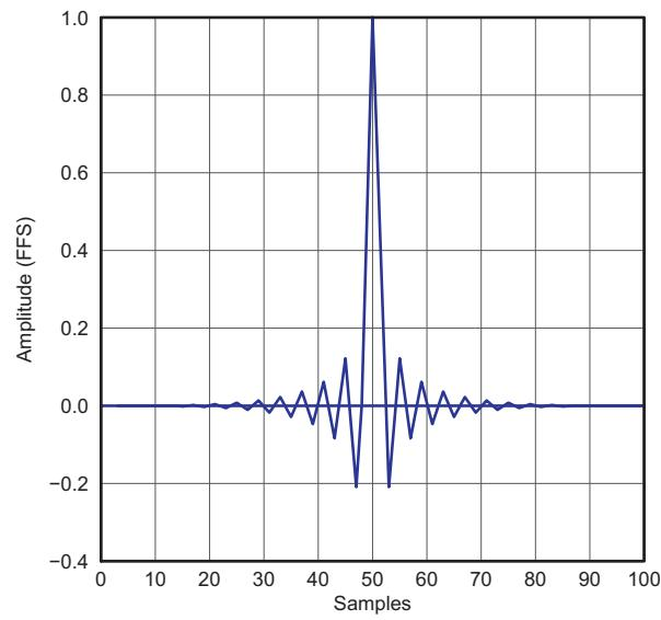
**Figure 26. Normal x2 Interpolation Filter Impulse Response**
