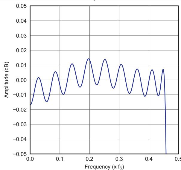
**Figure 21. Normal x8 Interpolation Filter Passband Ripple**
