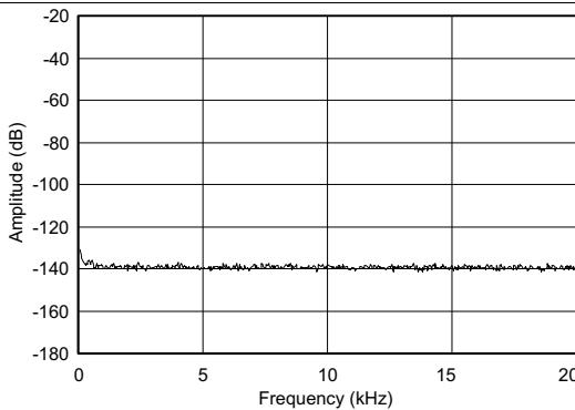
Figure 7. PCM5121 FFT Plot at Bipolar Zero Data (BPZ)
