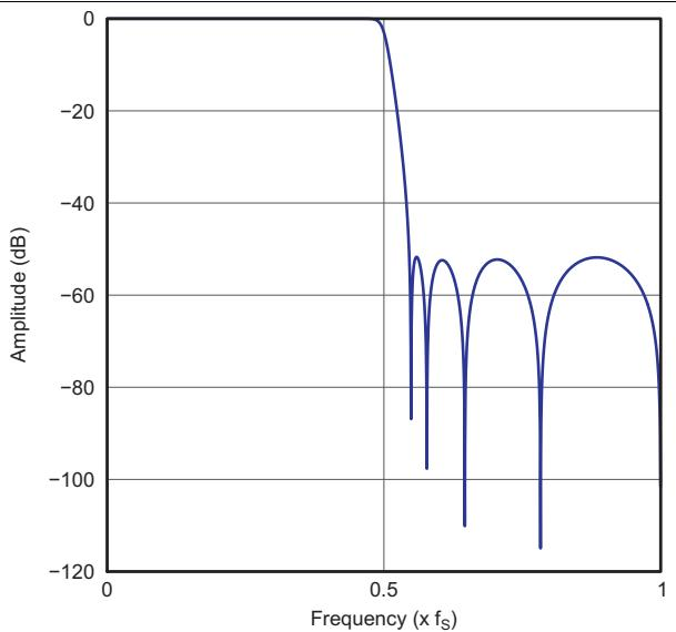
**Figure 34. Low Latency  $\times 2$  Interpolation Filter Frequency Response**
