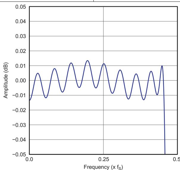
**Figure 24. Normal x4 Interpolation Filter Passband Ripple**
