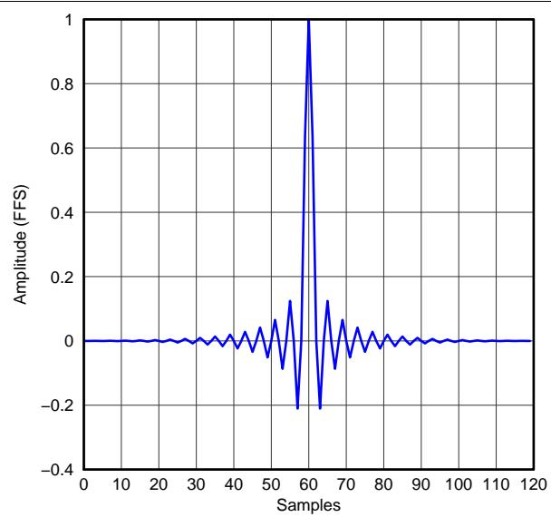
**Figure 53. High-Attenuation x2 Interpolation Filter Impulse Response, Quad Rate**
