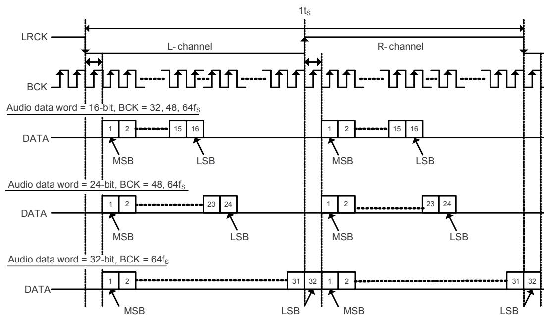
I<sup>2</sup>S Data Format; L-channel = LOW, R-channel = HIGHFigure 14. I<sup>2</sup>S Audio Data Format
