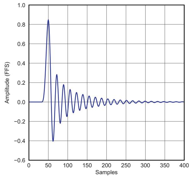
**Figure 29. Low Latency x8 Interpolation Filter Impulse Response**
