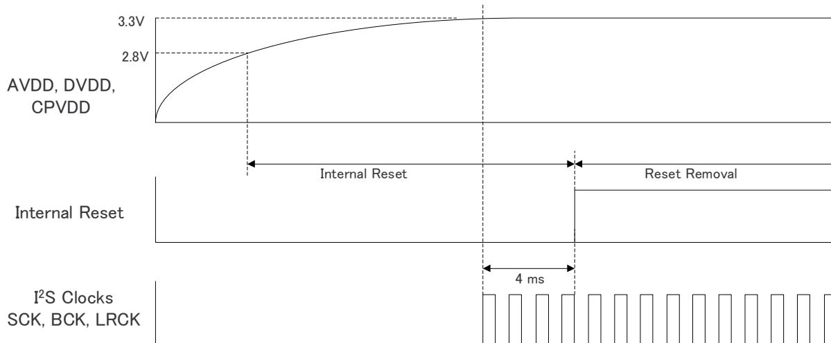
**Figure 83. Power-On Reset Timing, DVDD = 3.3 V**
