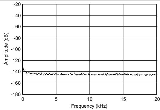
Figure 8. PCM5122 FFT Plot at BPZ
