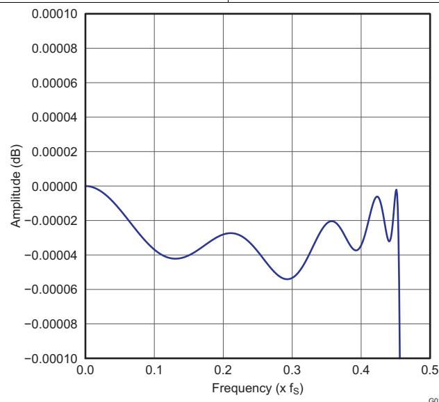
**Figure 30. Low Latency x8 Interpolation Filter Passband Ripple**
