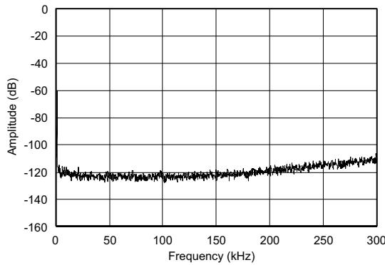
**Figure 11. PCM5121 FFT Plot Using a 1-kHz Tone (-60 dBFS) from DC to 300 kHz**
