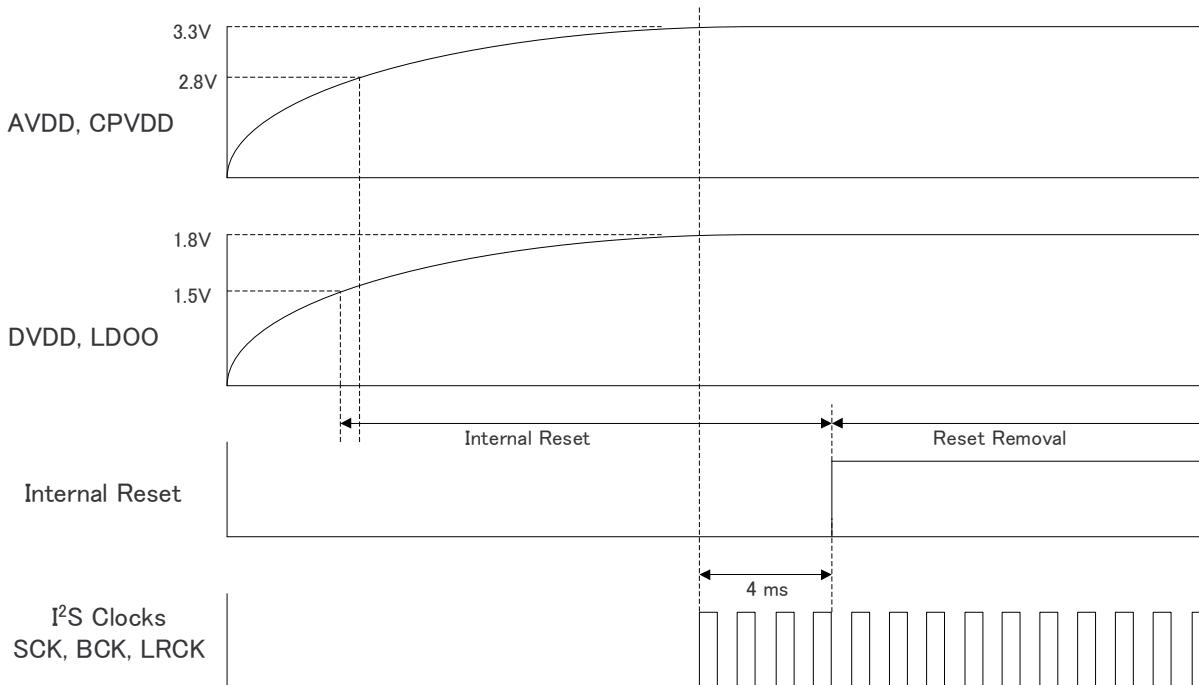
**Figure 84. Power-On Reset Timing, DVDD = 1.8 V**
