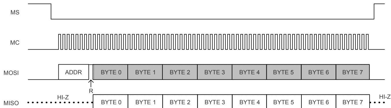
**Figure 70. Serial Control Format; Read, Multiple Byte**
