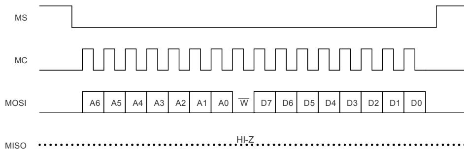
**Figure 67. Serial Control Format; Write, Single Byte**
