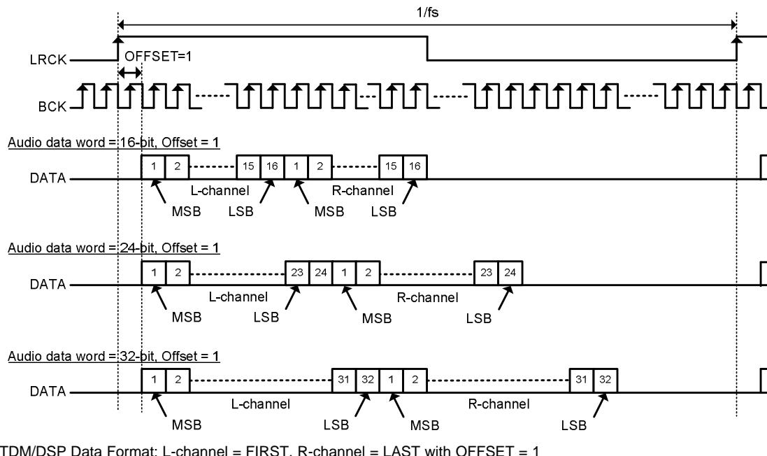
TDM/DSP Data Format; L-channel = FIRST, R-channel = LAST with OFFSET = 1
