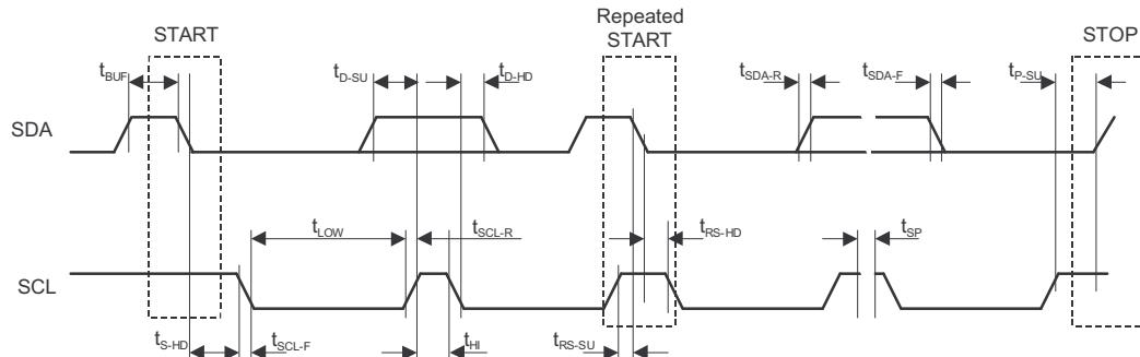
**Figure 74. Register Access Timing**
