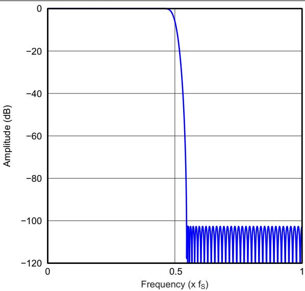
**Figure 52. High-Attenuation x2 Interpolation Filter Frequency Response, Quad Rate**
