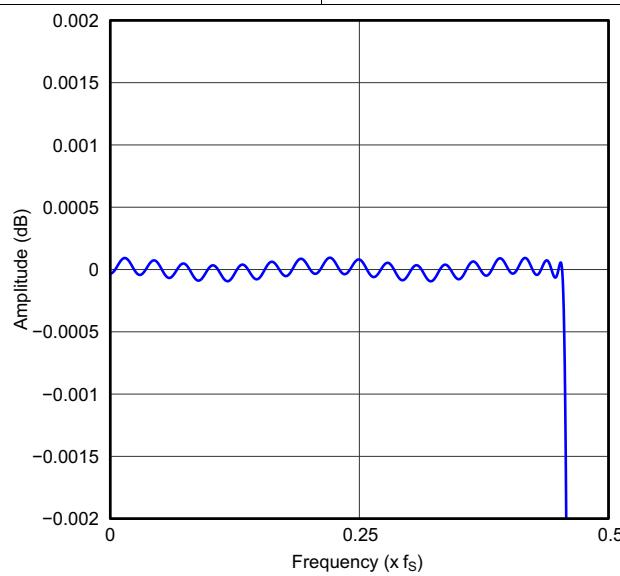
**Figure 51. High-Attenuation x4 Interpolation Filter Passband Ripple, Dual Rate**
