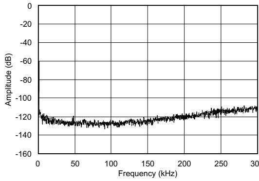
**Figure 12. PCM5122 FFT Plot Using a 1-kHz Tone (-60 dBFS) from DC to 300 kHz**
