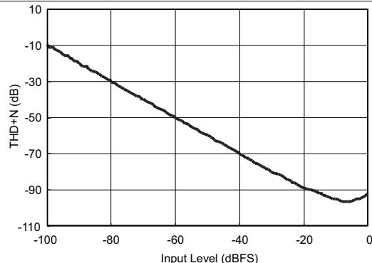
Figure 4. PCM5122 THD+N vs Input Level
