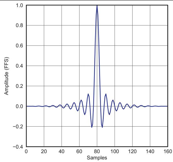
**Figure 23. Normal x4 Interpolation Filter Impulse Response**
