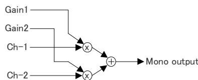
**Figure 60. Mono Mixer Block****Table 26. Mono Mixer Coefficients**
