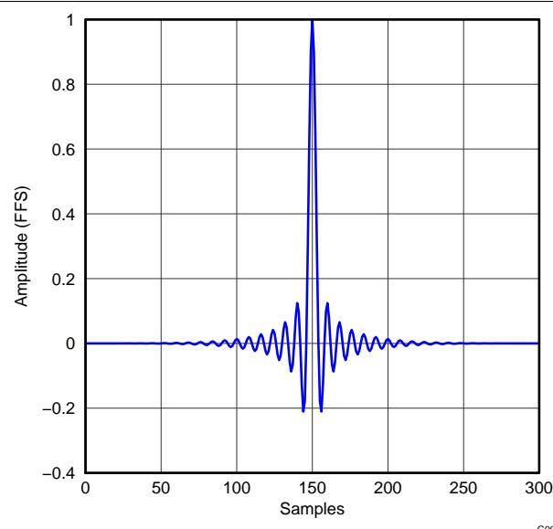
**Figure 50. High-Attenuation x4 Interpolation Filter Impulse Response, Dual Rate**
