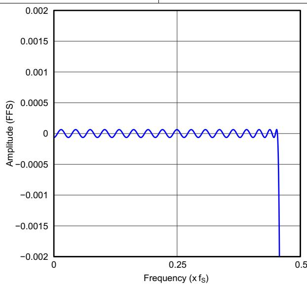
**Figure 54. High-Attenuation x2 Interpolation Filter Passband Ripple, Quad Rate**
