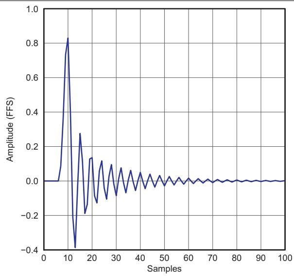
**Figure 35. Low Latency  $\times 2$  Interpolation Filter Impulse Response**
