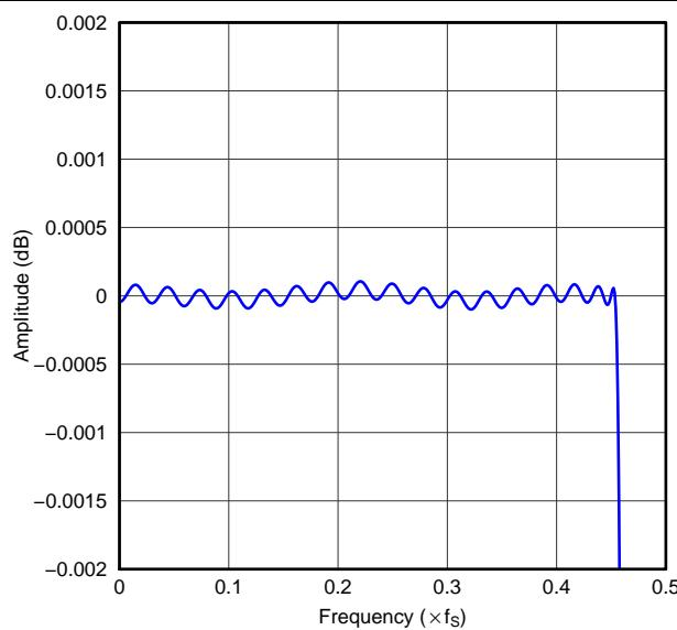
**Figure 48. High-Attenuation x8 Interpolation Filter Passband Ripple, Single Rate**
