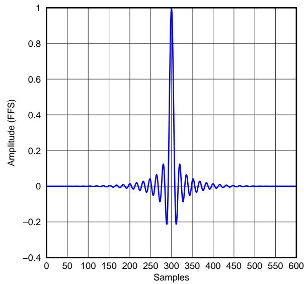
**Figure 47. High-Attenuation x8 Interpolation Filter Impulse Response, Single Rate**
