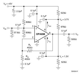
Figure 48. AC-Coupled, Single-Supply Amplifier
