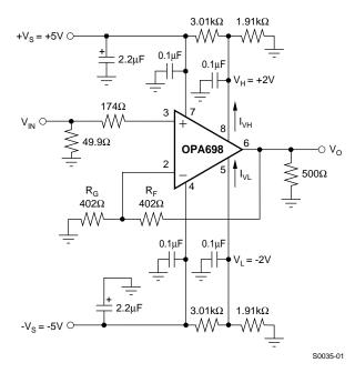
Figure 47. DC-Coupled, Dual-Supply Amplifier
