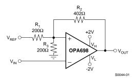
Figure 61. High-Speed Schmitt Trigger
