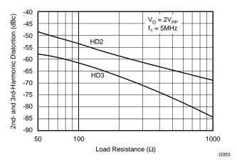
Figure 69. 5-MHz Harmonic Distortion vs Load Resistance
