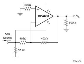
Figure 55. High-Speed Full-Wave Rectifier #1
