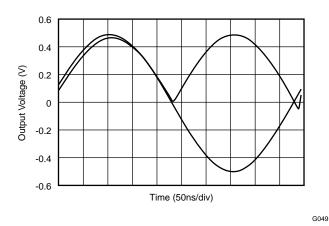
Figure 56. 2-MHz Sinewave Rectified
