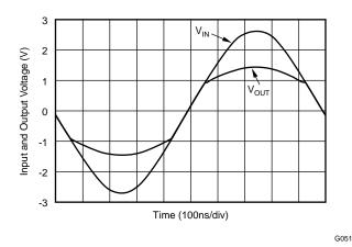
Figure 60. Soft-Clipping With A Gain of 1/3 Above the Clamp Level (±1 V)
