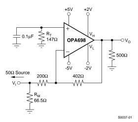
Figure 49. Inverting G = -2 Specifications and Test Circuit
