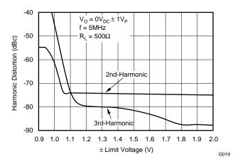
Figure 67. Harmonic Distortion Near Limit Voltages
