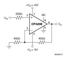
Figure 53. Precision Half-Wave Rectifier
