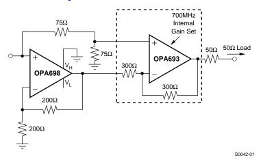
Figure 57. High-Speed Full-Wave Rectifier #2
