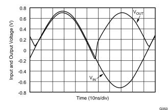
Figure 58. 10-MHz Sinewave Rectified
