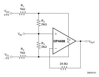
Figure 59. Soft-Clipping Circuit
