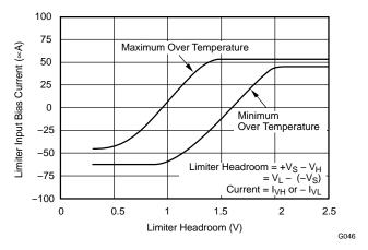
Figure 66. Limiter Bias Current vs Bias Voltage
