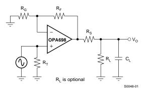
Figure 68. Driving Capacitive Loads
