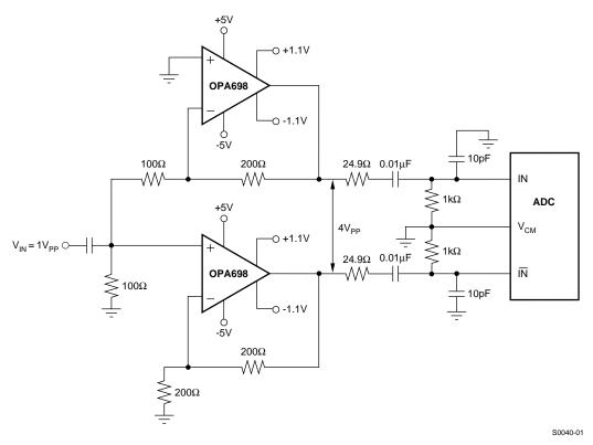
Figure 52. Single-to-Differential AC-Coupled, Output Limited ADC Driver
