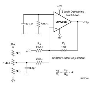
Figure 71. DC-Coupled, Inverting Gain of -2, With Offset Adjustment
