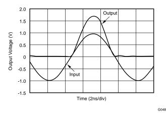
Figure 54. 100-MHz Sine Wave Rectified
