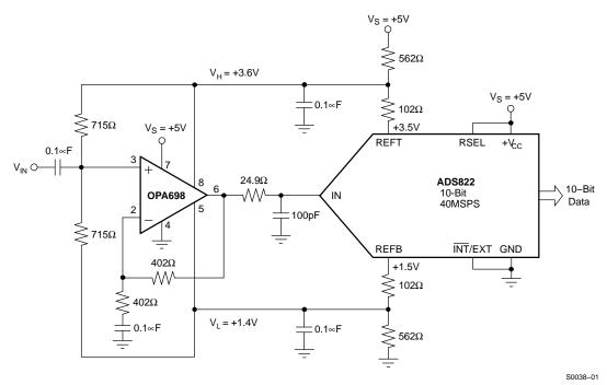
Figure 51. Single Supply, Limiting ADC Input Driver
