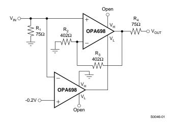
Figure 65. Sync Stripper Circuit
