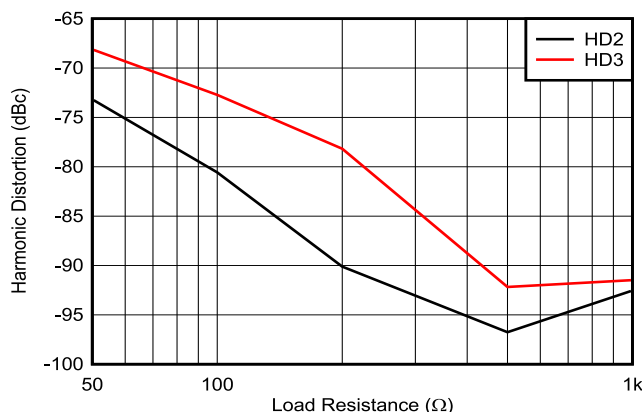
Figure 8-4. 5MHz Harmonic Distortion vs Load Resistance
