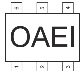
Figure 5-2. DBV Package, 6-Pin SOT-23 (Top View)
